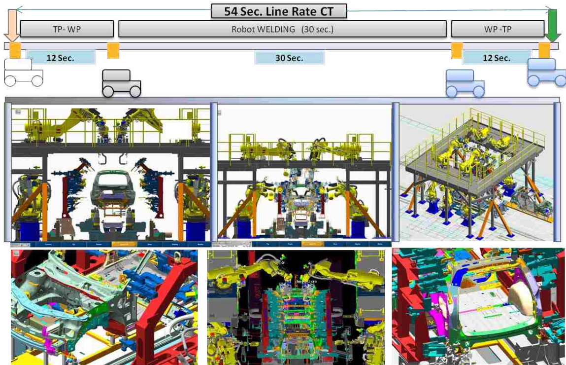
Fig. 3- 18: Vehicle framing; Open-Gate system complete cycle
