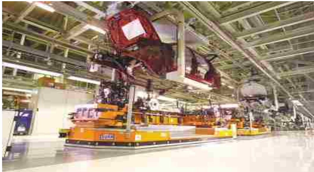
Fig. 2- 8: Car body marriage over power train and rear axle trolleys
