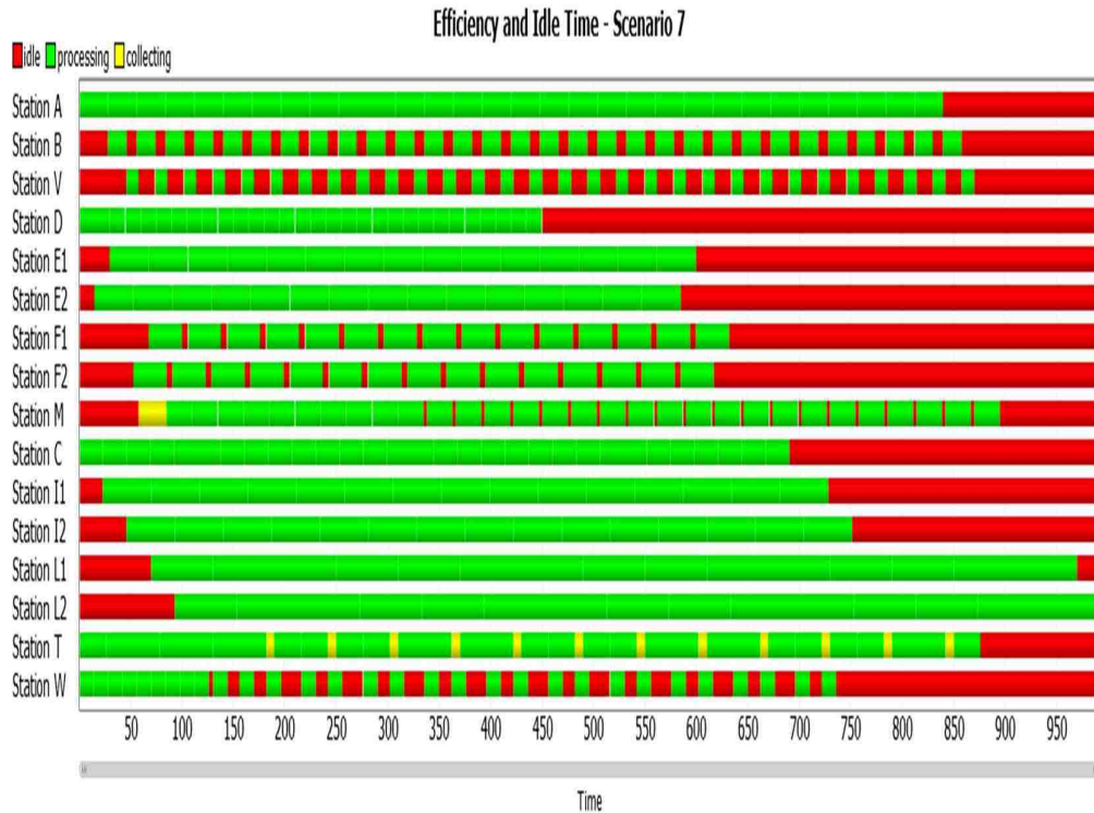
Figure 5.14 FlexSim Gantt Chart for Scenario 7, Four Parallel Station at E, F, I, and L Plus Two Buffers at T and W
