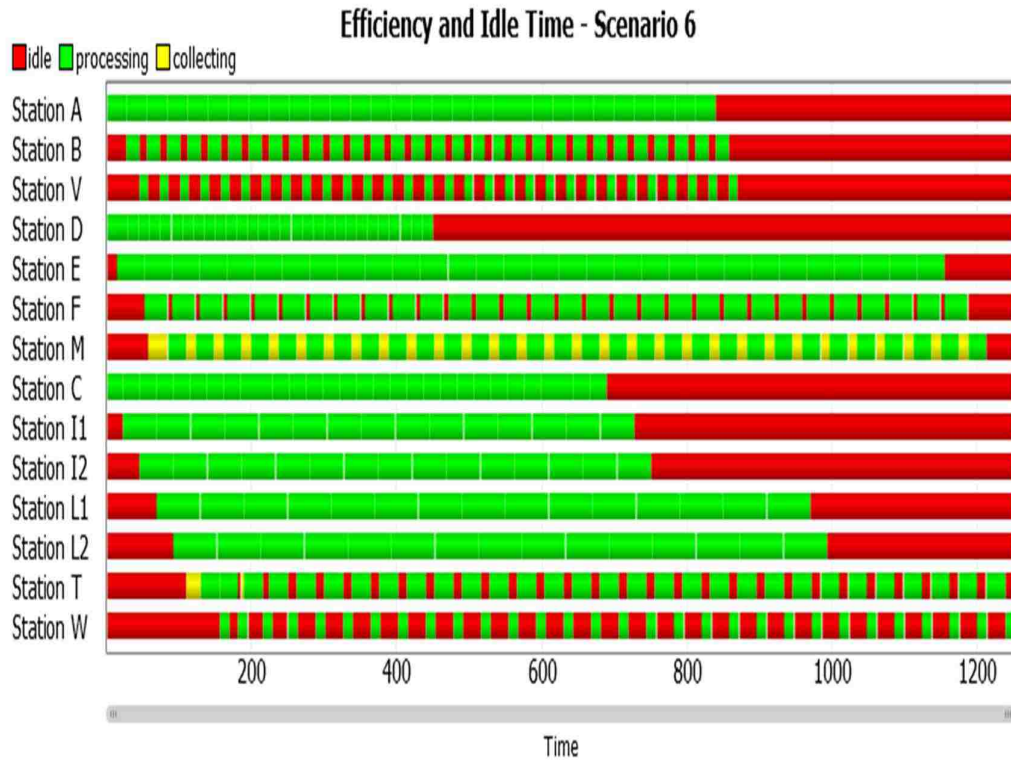
Figure 5.12 FlexSim Gantt Chart for Scenario 6, Two Parallel Stations at I and L
