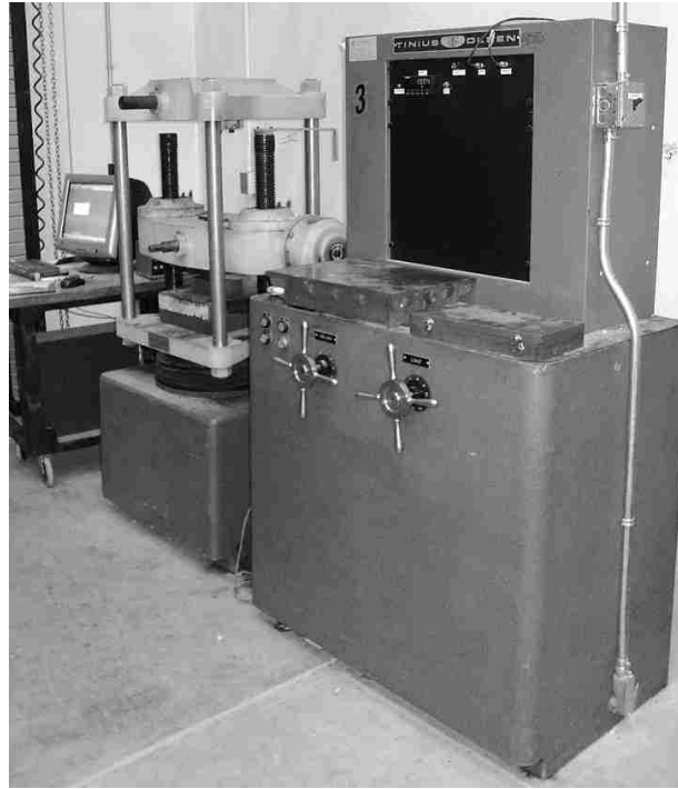
Figure 5.3. 1Tinius Olsen® tensile/compressive equipment setup
