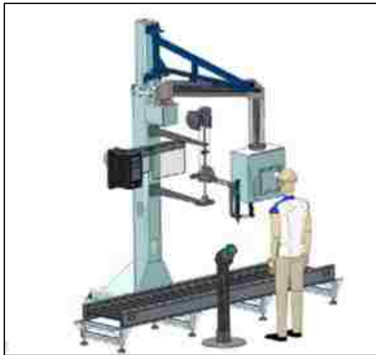
Figure 1.3: Typical Manual Work Station used in assembly line
