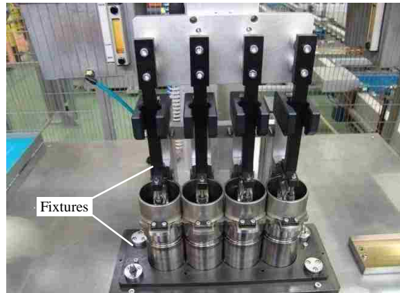
Figure 5.8: Insertion of the piston-rod sub-assembly into the cylinder liners at station 6
