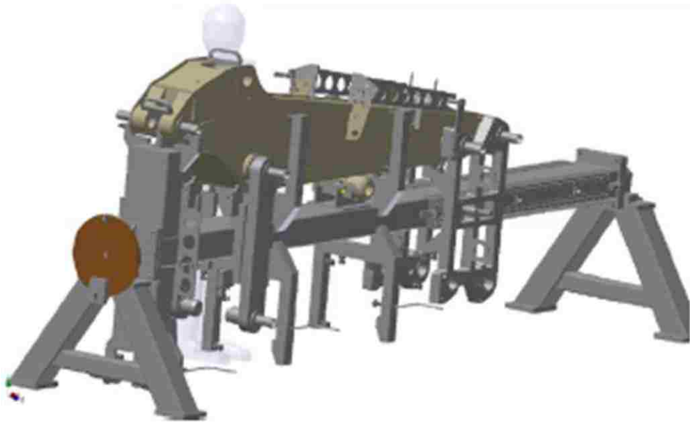
Figure 4.1: Example of one of the existing, dedicated tack-welding fixtures subject to the case study presented by Bejlegård et al. (2018)
