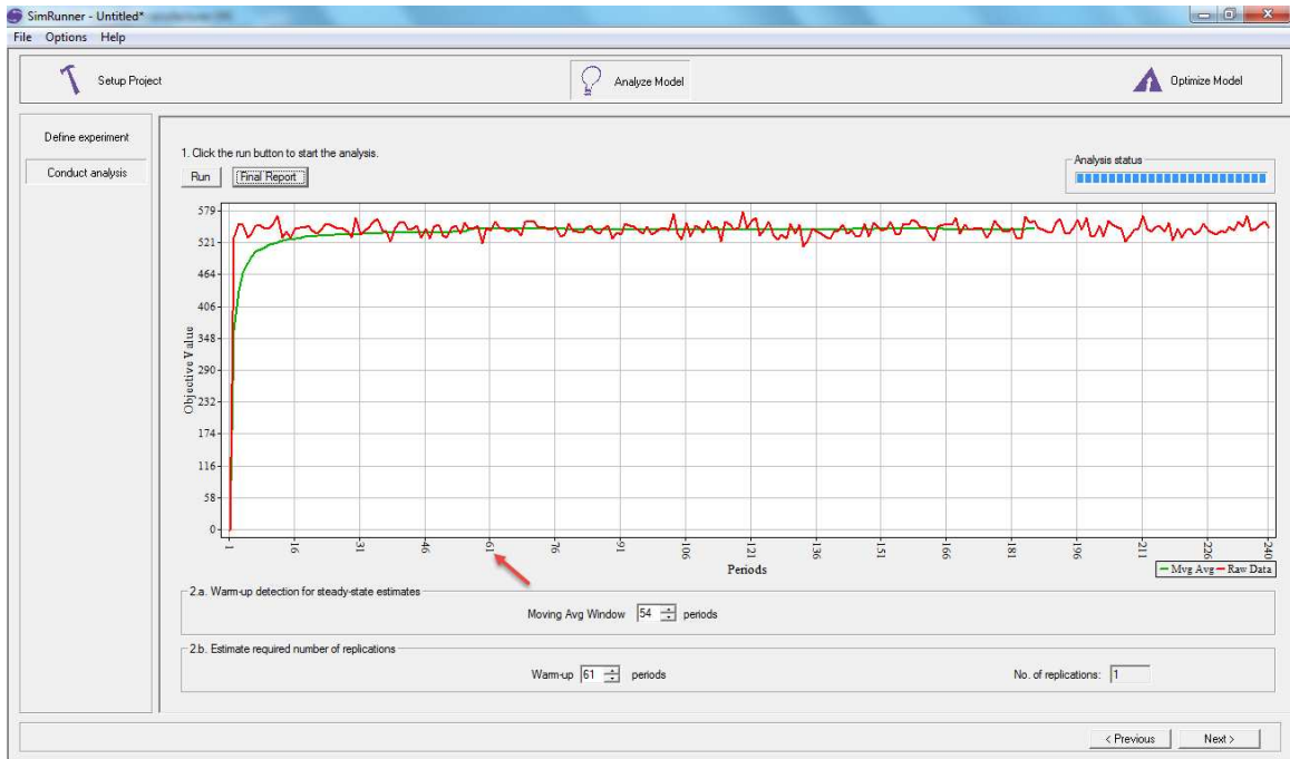
Figure 31: Warm-up Period Graph: Moving average plot for moving average window, w = 54
