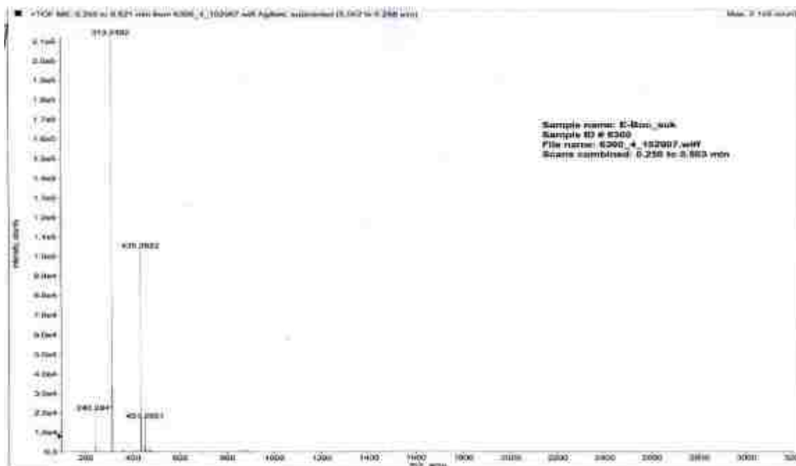
Appendix I-A. Electrospray Ionization mass spectrum of \epsilon -Boc-SUK. The peak at 435 amu is representative of \epsilon -Boc-SUK.
