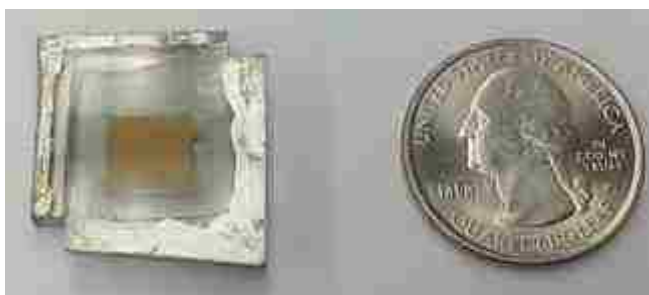
Figure 4.4 Photograph image of a fabricated DSSC with use of a quarter as a scale.
