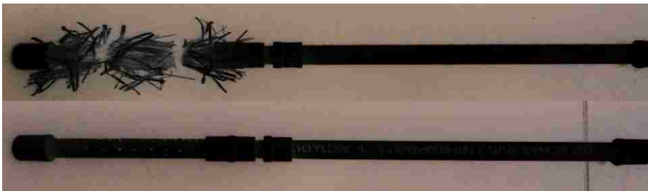
Figure 2. Photograph of the nutrient diffusion system constructed for this study with grass leaves attached on the left and just the diffusion tube on the right, the longer PVC pipe acted as the reservoir for the nutrient enriched water.
