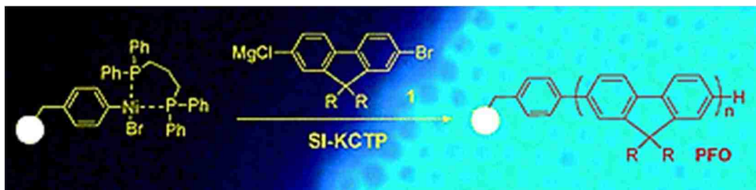
Figure 1.10: Grafting of PFO from microparticles via SI-KCTP. Reproduced with permission from ref. 76. Copyright © 2010 Royal Chemical Society.
