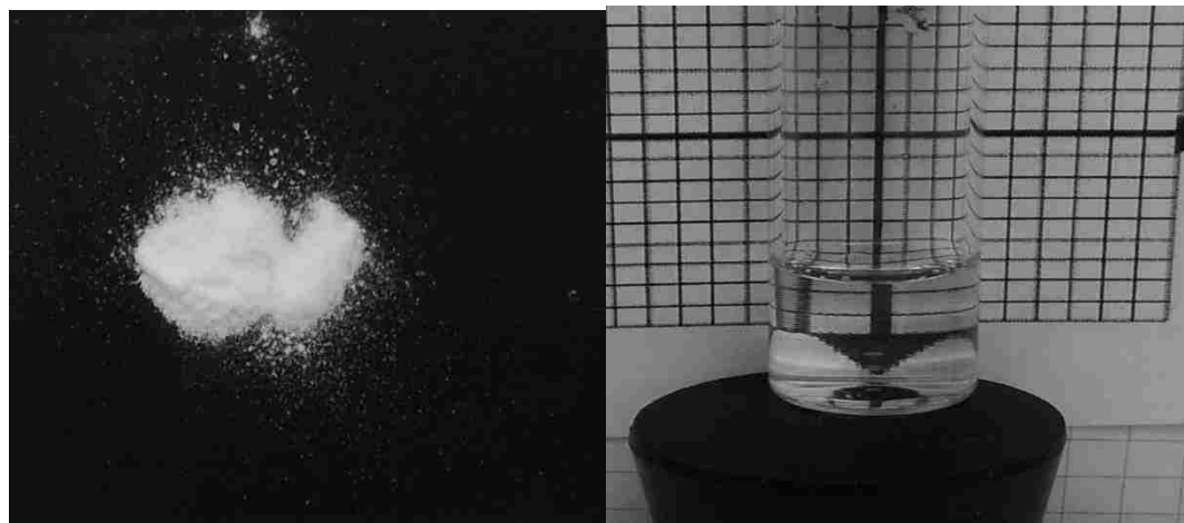
Fig. 4. Polymer 3 CUP dried and powdered (left) and re-dissolved/dispersed (right) in water
