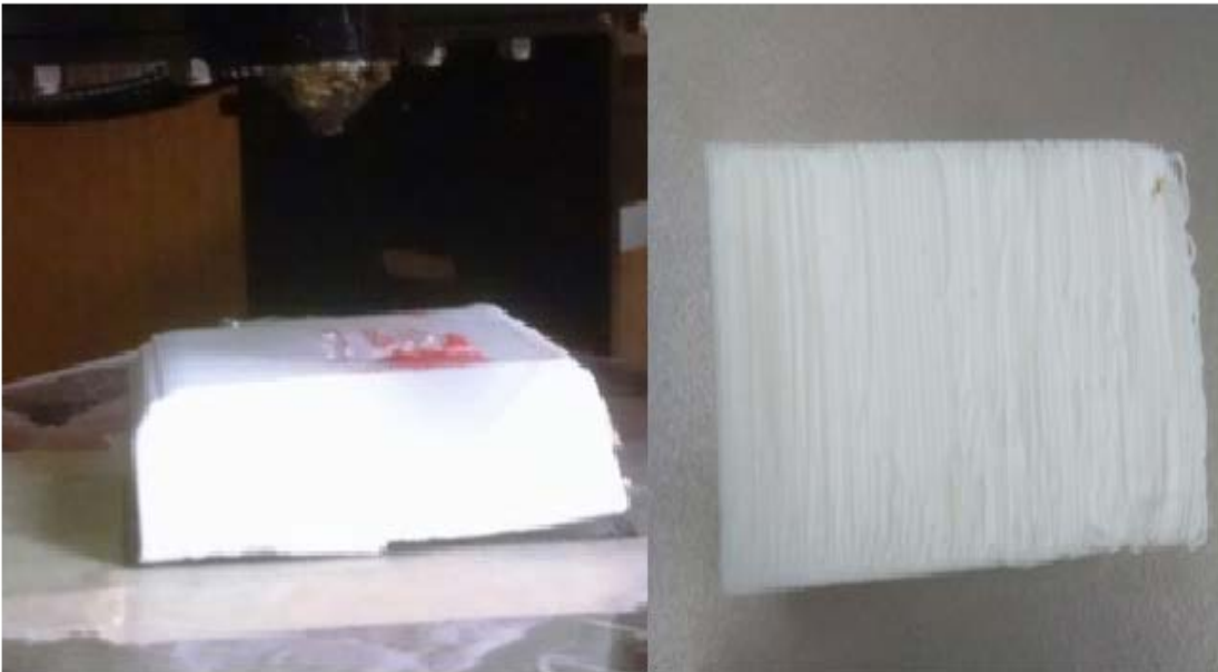
Figure 4.10. Unevenness when substrate is printed at 45 ° relative to the X-axis
