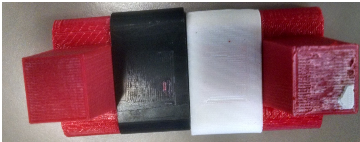
Figure 4.7. Interface of the substrate and auxiliary part after tensile testing
