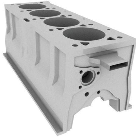
Figure 1: The figure show an example of a complex part containing holes, pockets, sharp corners, and protrusions. [18]
