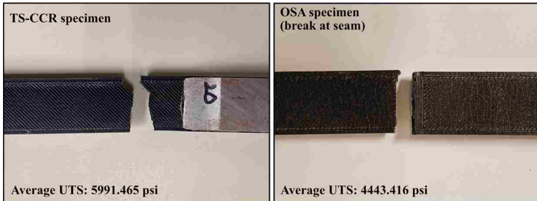
Figure 4.3. Fractures of specimens printed by two different methods.
