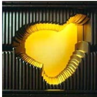
Figure 1.3: Modulating a Beam by a Multi-leaf Collimator
