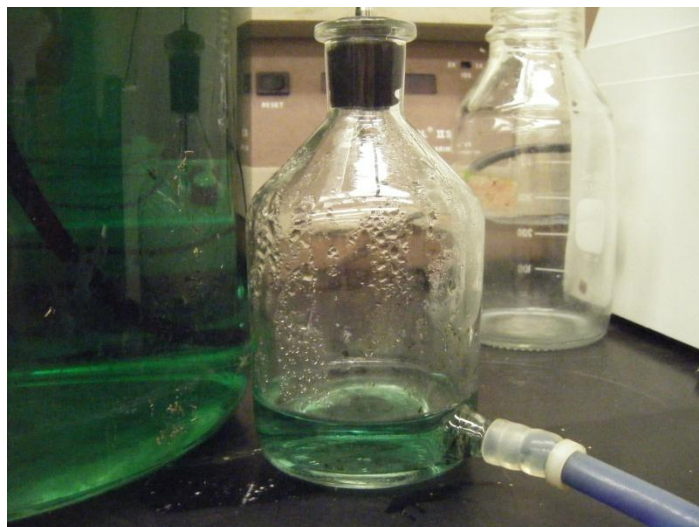
Figure 5 Airlock used to avoid back-contamination of media reservoir
