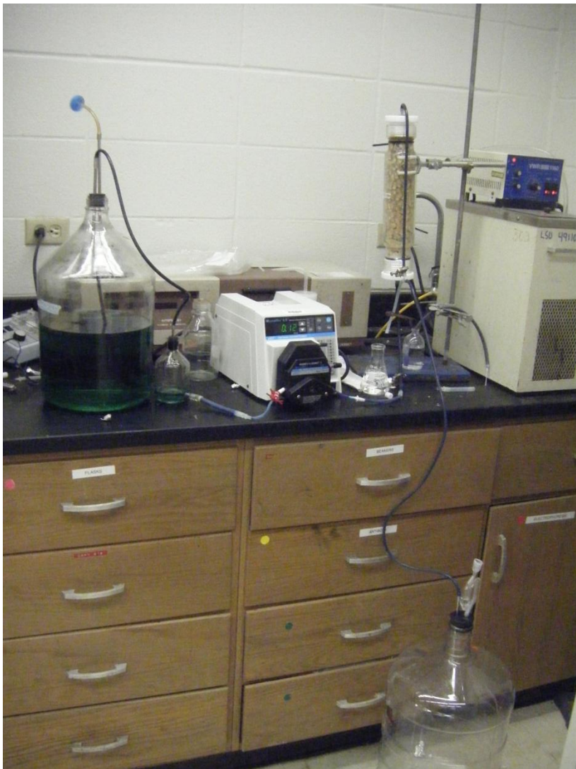
Figure 4 Immobilized culture apparatus flowing with 3.5% glucose medium. Silicon tubing, 0.0625" I.D. x 0.125" O.D. inside 0.125" I.D. x 0.25" O.D. near the pump and 0.188" I.D x 0.313" O.D. around the rest of the apparatus was used
