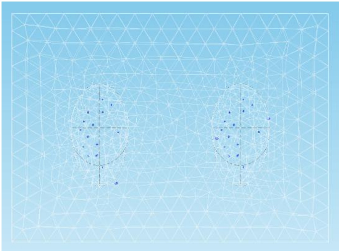
Figure 5.5 (b) Cold spots (blue area) in the unsealed meal paste and oyster meat after heating
