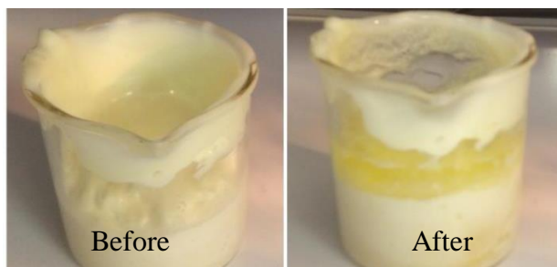
Figure 4.7 Emulsion stability before and after a failed heat stability test
