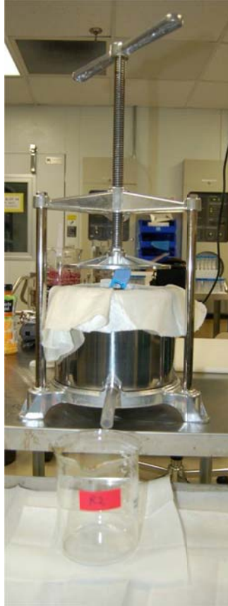
Supplemental Image A.1 Stainless steel press showing nylon press cloth and spigot for juice extraction.
