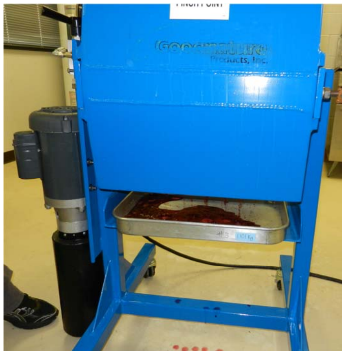
Supplemental Image A.4 Pilot scale pressing of rabbiteye 'Tifblue' blueberries in a Goodnature X-1 press, showing the juice flowing out the bottom of the press into a stainless steel pan.
