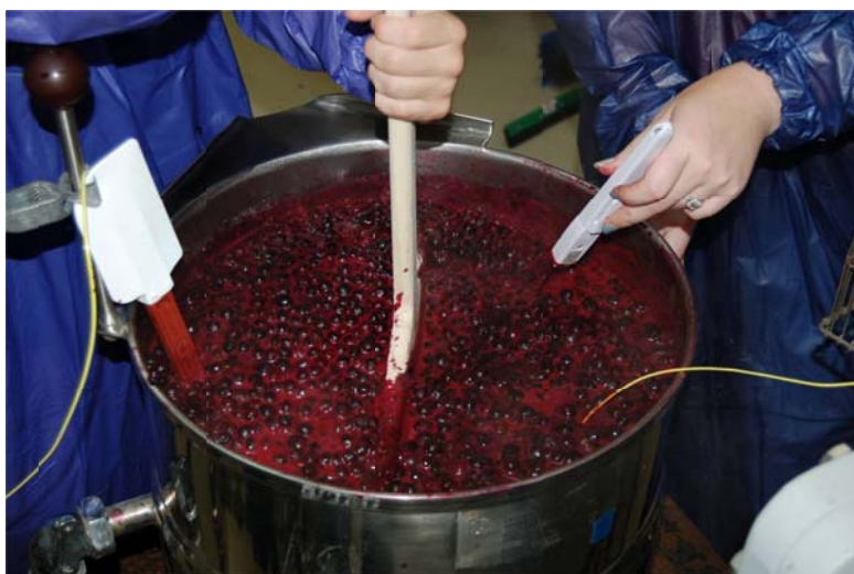
Supplemental Image A.3 Pilot scale steam jacketed kettle mashing of rabbiteye 'Tifblue' blueberries heated to 95 °C with constant stirring.
