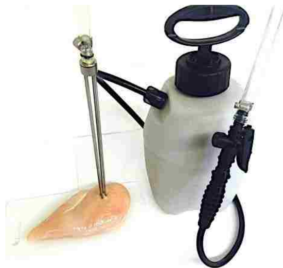
Figure 2. Manual injector and a 4-needle set attached used to inject chicken breasts (Model 5318 Home 1 gallon sprayer, Project Source™ Cincinnati, OH).
