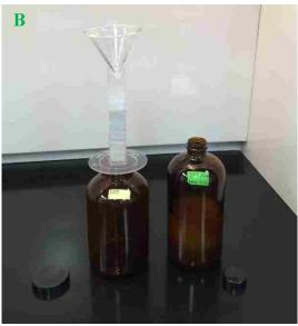
Figure 4.1 (A) Water filtration system (B) Filtration of surface water through natural zeolite and HDTMA-Cl SMZ.
