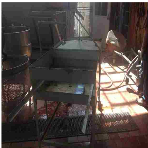
Figure 4. A Picture of the Vegetable Blancher used to Steam the Live Crawfish
