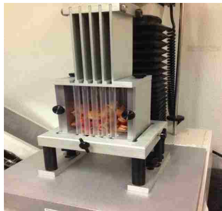
Figure 6. Texture Analyzer with a 5-blade Kramer Attachment used for Simultaneous Measurement of Shear Force and Work of Shearing.
