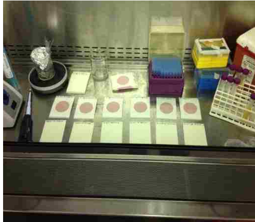
Figure 5. Hood and Petrifilms used for Coliform (Above/Red) and Aerobic (Below/Yellow) Counts.
