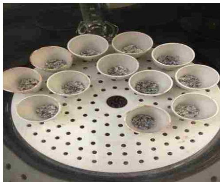
Figure 7. Samples in Ceramic Crucibles after Moisture Analysis and Subsequent Ashing.
