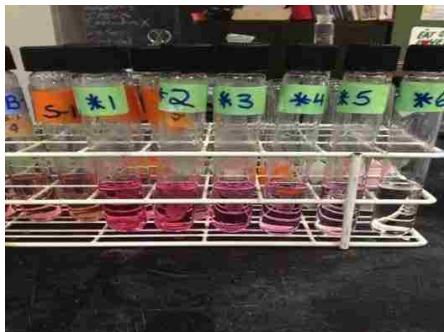
Figure 9. Test Tube Holder Containing the Standard Curve (*1-*6) Solutions and Test Samples Behind (S-1, etc.) for TBARS Analysis.
