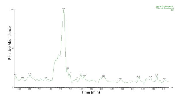
Figure 3.4: Extracted ion chromatogram for enrofloxacin in sample 2
