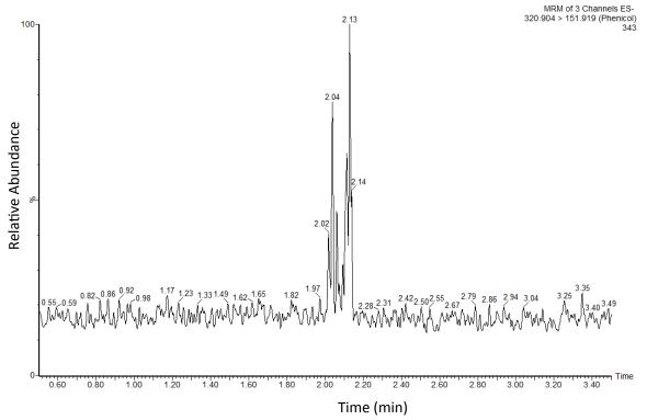
Figure 3.1: Extracted ion chromatogram for chloramphenicol in sample 1
