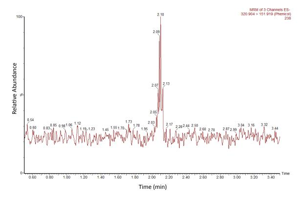
Figure 3.3: Extracted ion chromatogram for chloramphenicol in sample 4
