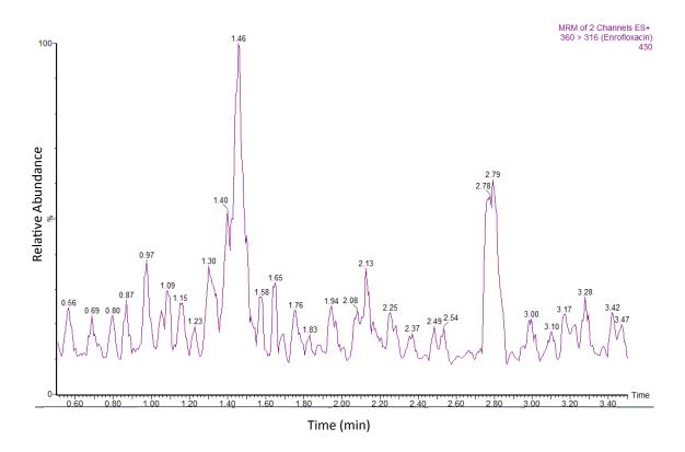
Figure 3.5: Extracted ion chromatogram for enrofloxacin in sample 3
