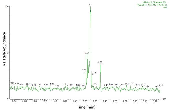
Figure 3.2: Extracted ion chromatogram for chloramphenicol in sample 2
