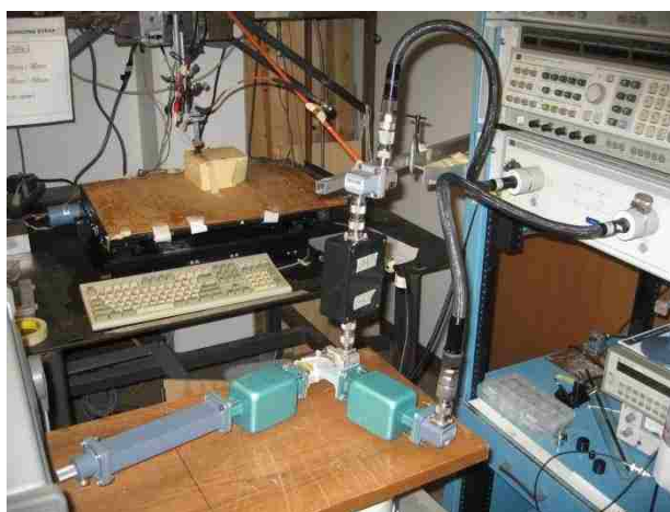
Figure 5.18. System orientation during the characterization process illustrating cable stresses.
