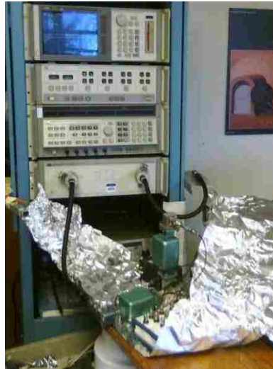
Figure 5.24. Metal foil for ground-noise removal.
