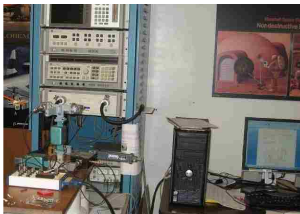
Figure 5.25. Setup to perform measurements using a Magic-T.
