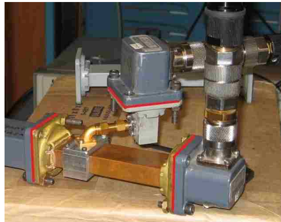
Figure 2.2. RF Coupler for the X-band VNA with the three waveguide reference planes marked in red (old design).
