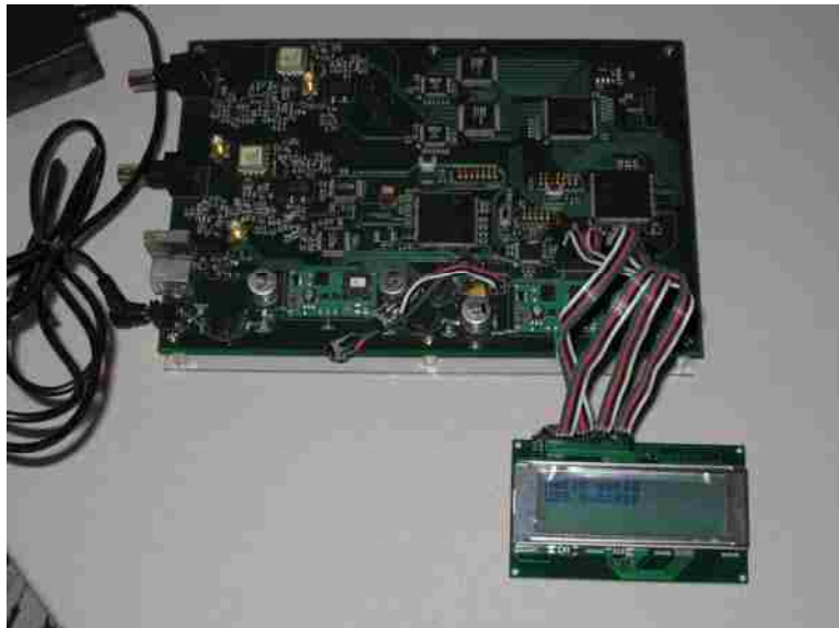
Software Defined Radio with LCD Display
