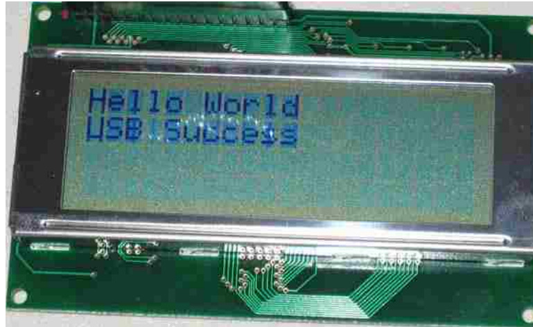
Figure 3.10: Successful LCD Display Test
