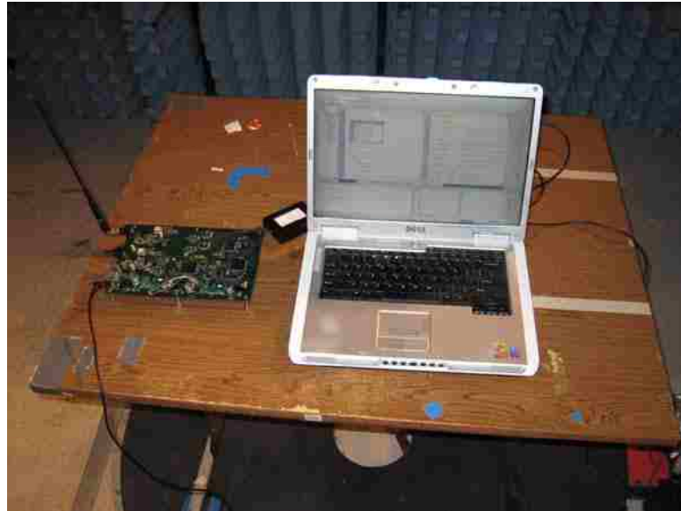
Transmitter Test Setup: SDR Setup
