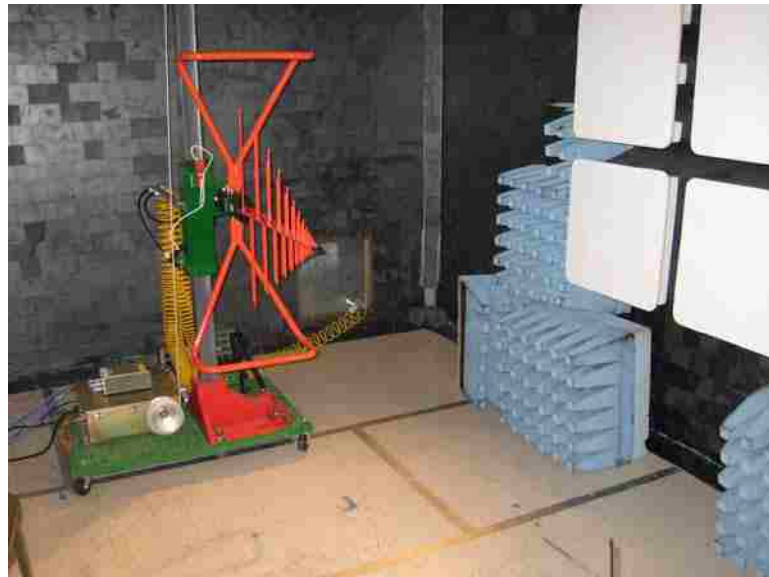
Transmitter Test Setup: Semi-Anechoic Chamber
