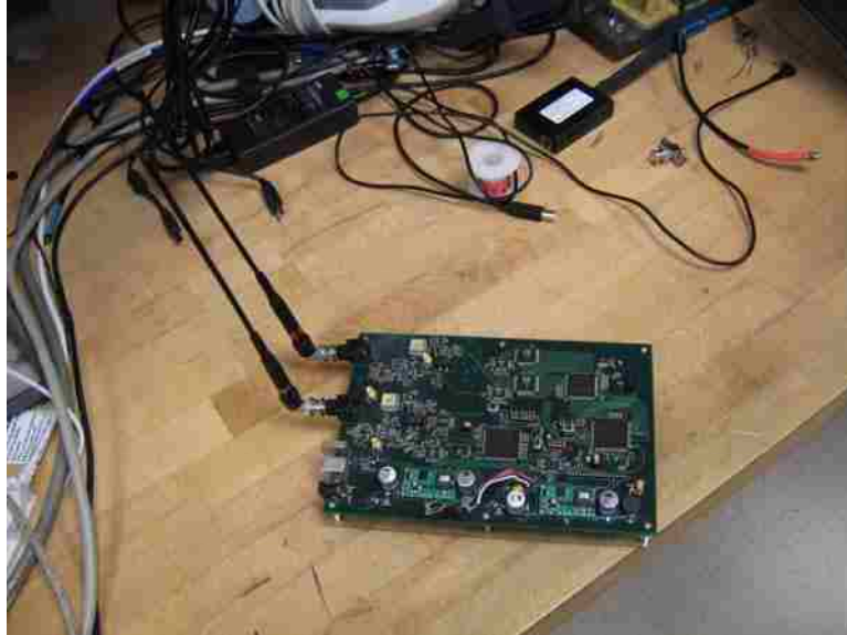
Software Defined Radio with Antennas
