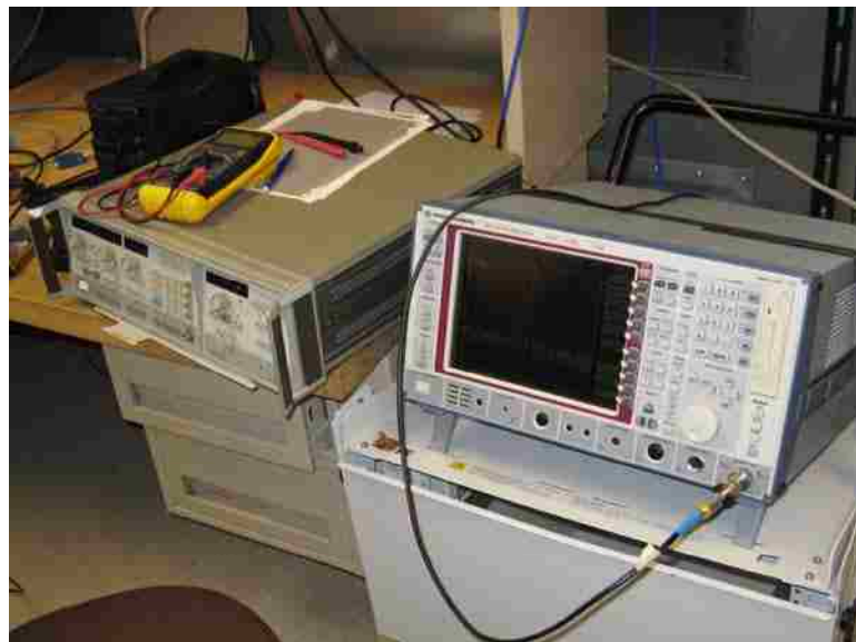
Transmitter Test Setup: Spectrum analyzer
