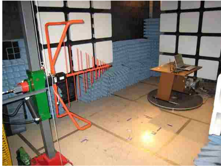
Transmitter Test Setup: Semi-Anechoic Chamber
