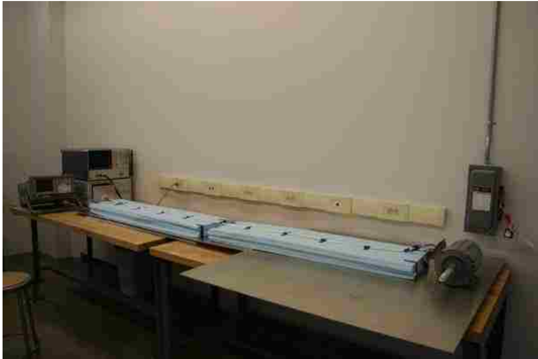
Figure 23 - Motor and Cable Test Setup: Full View
