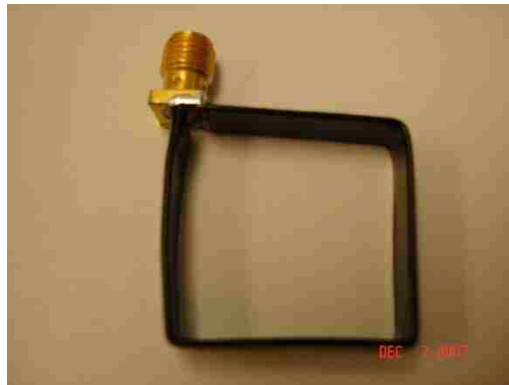
Figure 4.2. Copper Strap Wrapped in Electrical Tape
