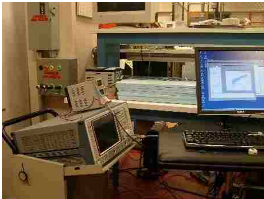
Figure 34 - Emissions Test Setup: Motor Drive, Spectrum Analyzer, Amplifier, and Current Probe
