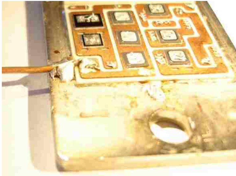
Figure 2.22. Measurement Setup for Area Fill B Capacitance
