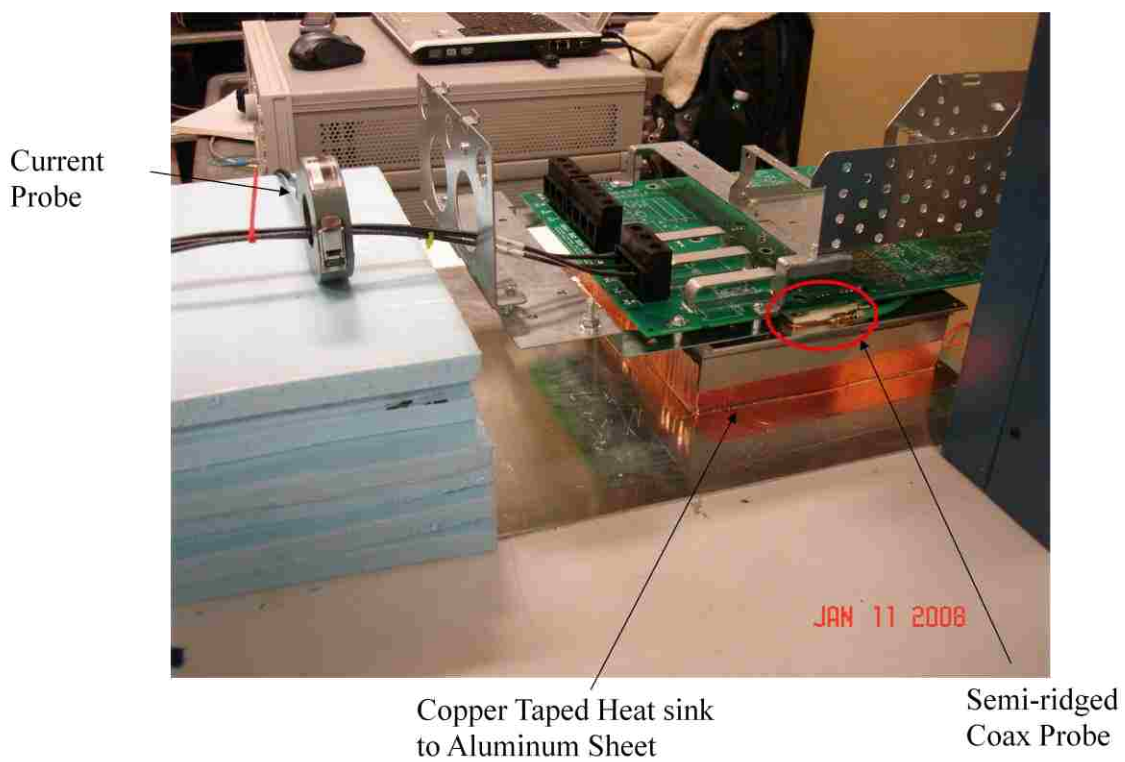
Figure 4.14. Setup for Transfer Impedance from IGBT to Cables Leading to the Motor
