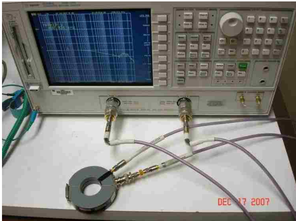
Figure 4.5. Current Probe Transfer Impedance Measurement Setup
