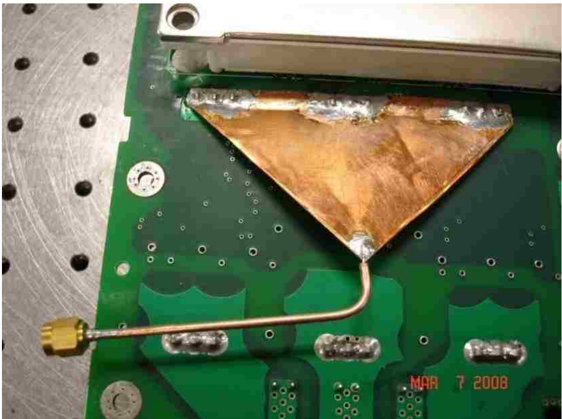
Figure 4.17. Copper Triangle Used to Connect the Center Conductor to the Three Phases and Reduce Inductance
