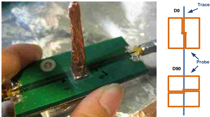
Figure 3-38. D0 response and D90 rejection measurement setup
