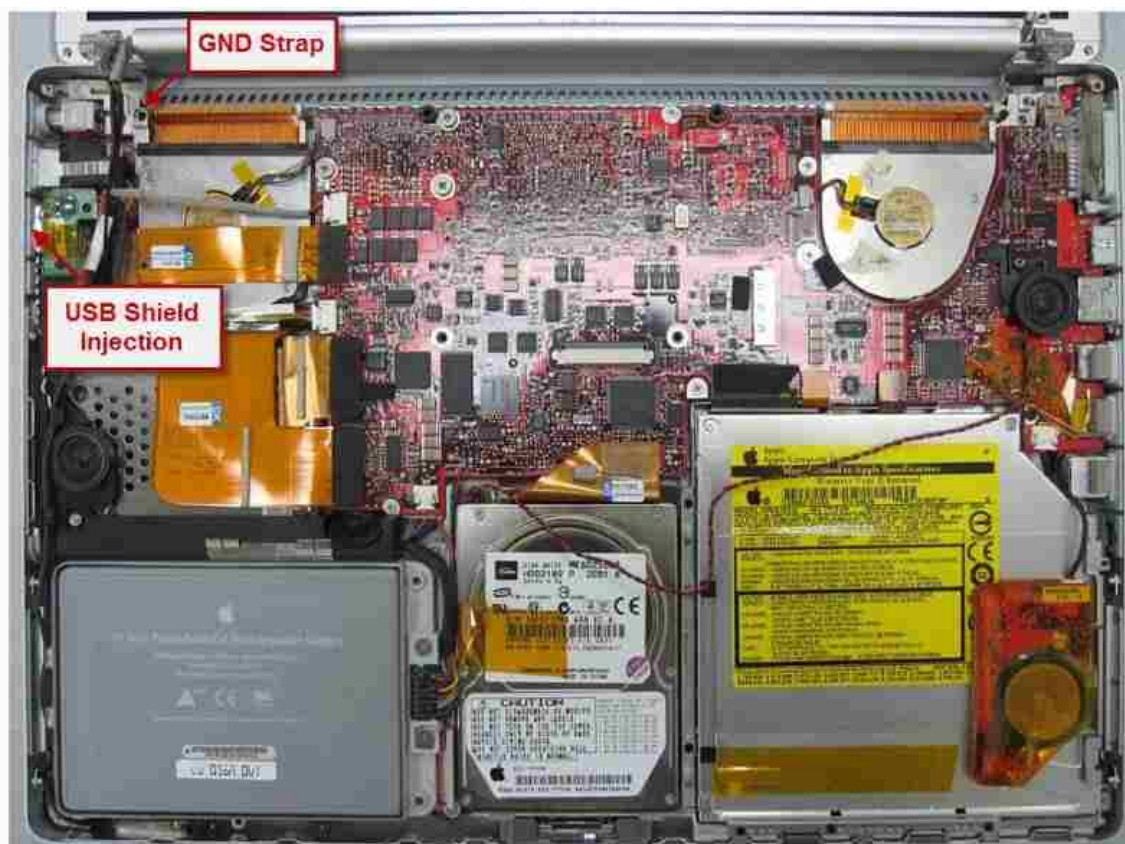
Figure 6-2 Injection location and ground strap connection at the Macbook
