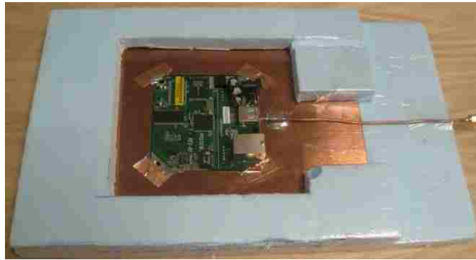
Figure 6-13. Printer server prepared for double side scanning
