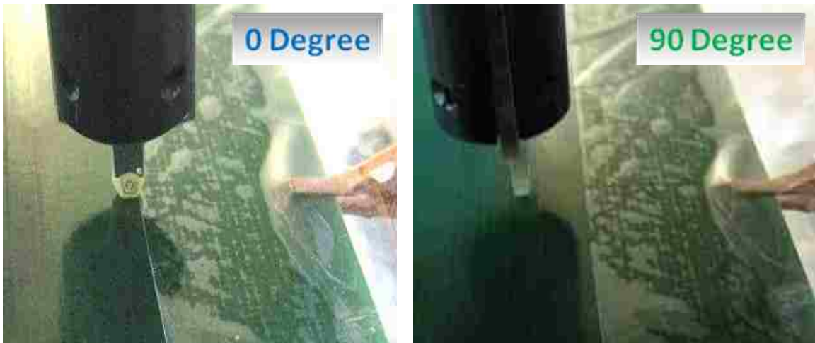
Figure 3-10. Unshielded probe in max and min H-field coupling orientations
