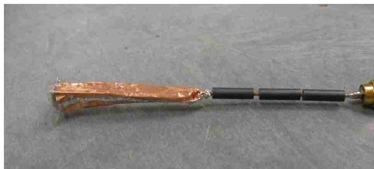
Figure 3-32. Assembled differential H_z probe
