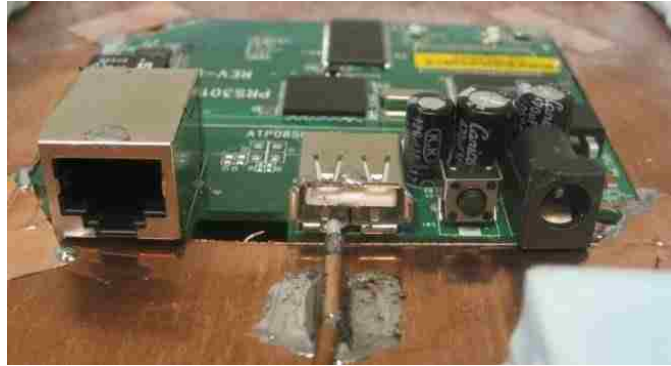
Figure 6-12. Injection location of printer server
