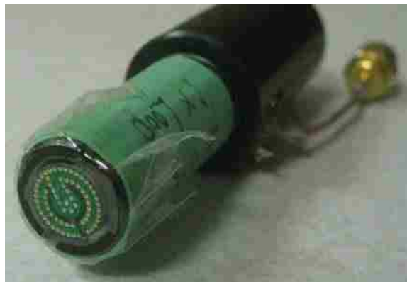
Figure 6-3. Shielded H_z field probe for near-field scanning
