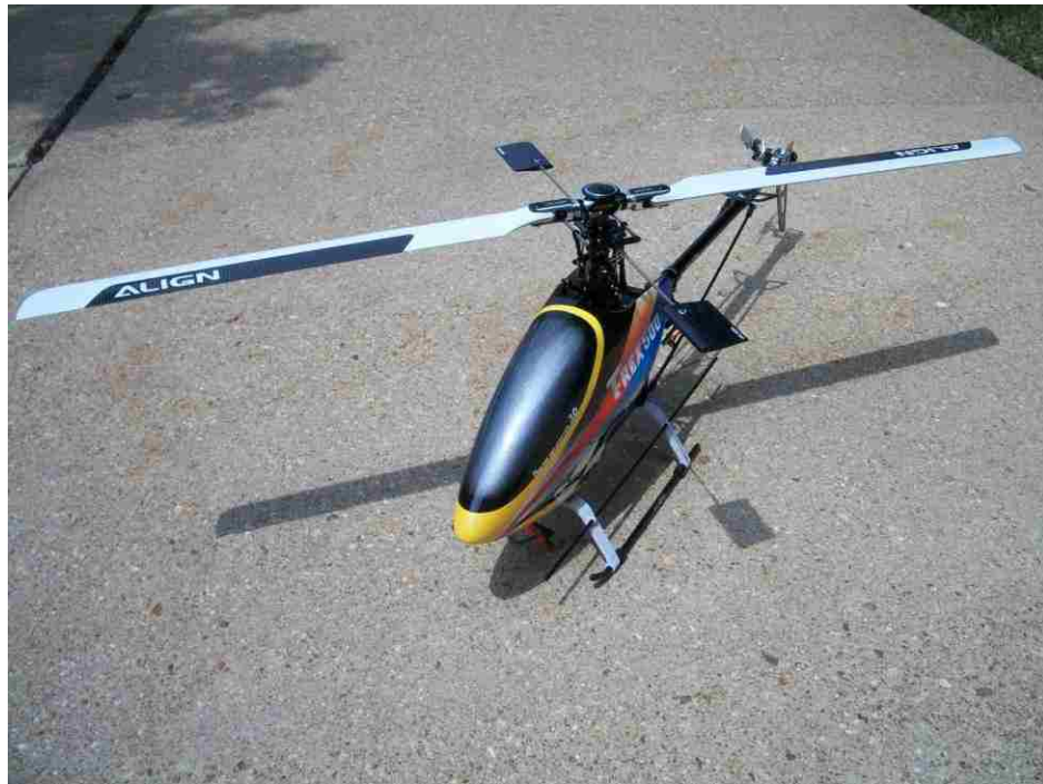
Figure 1.1. Helicopter UAV Built from Modified Align Trex 500 Airframe
