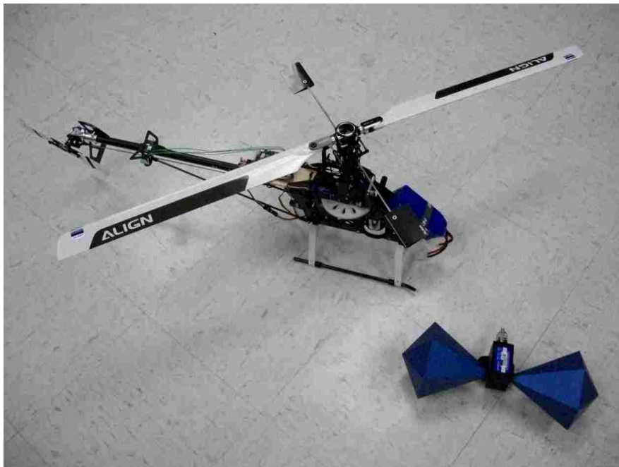
Figure 1.2. Helicopter UAV with Antenna for Threat Detection
