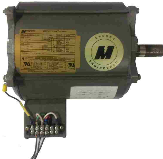
Figure A.7 Induction Machine – II Load
