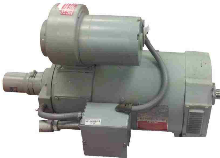
Figure A.2 DC machine (Prime-mover)
