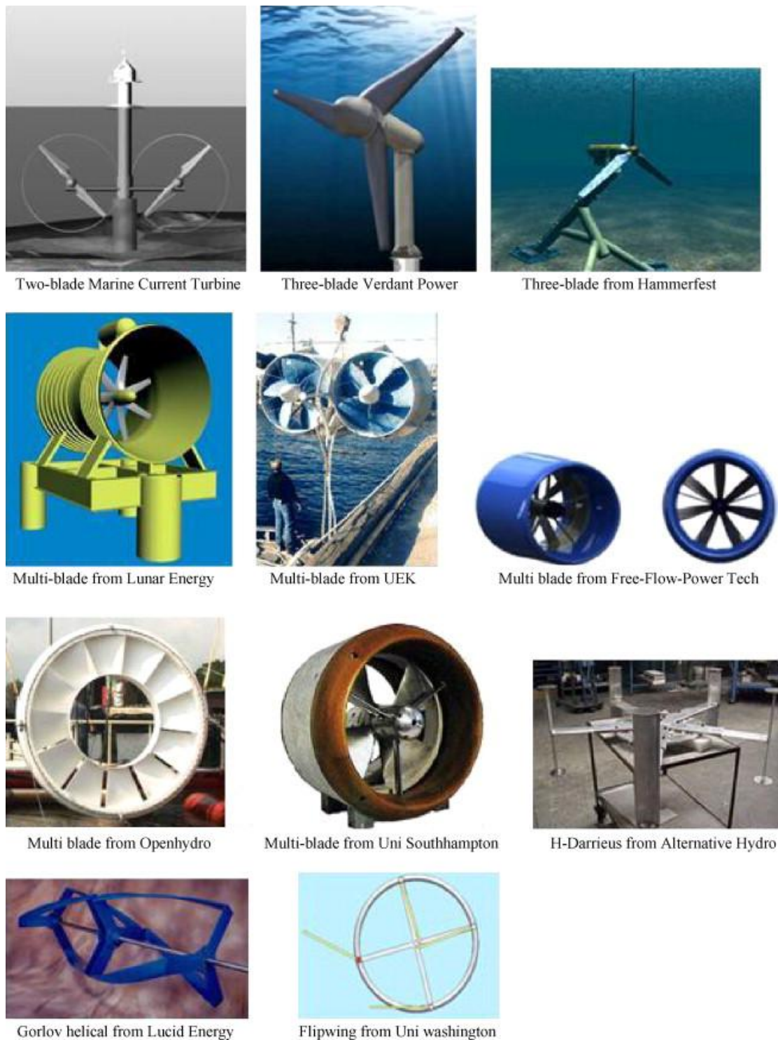
Figure 1.6: Sample of different configurations and concepts of hydrokinetic turbines explored at various institutions [15]
