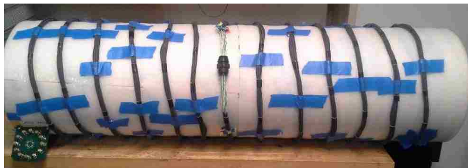
Figure 3.15. Measurement setup for Leoni Dacar 546 cable bundle with an inline CPC with maximum 25 cm untwisted segment
