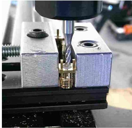
Figure 5.2. Milling process for removing SMA GND pins
