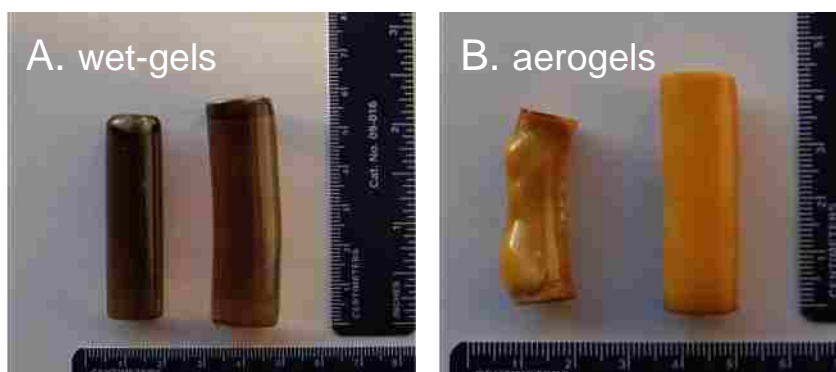
Figure 2. Photographs of: (A) a pDCPD-30 wet-gel immediately after removed from the mold (left) and of a similar gel swollen after 4 toluene washes (~32 h in toluene baths – right). (B) a pDCPD-30 aerogel (left-deformed) and of a pDCPD-30-X-MMA-50 aerogel (right).
