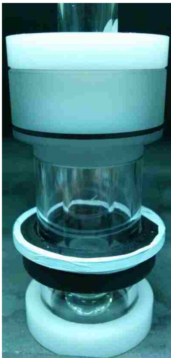
Figure 88. Adapter to use DLS cells in the Wyatt GPC detector.
