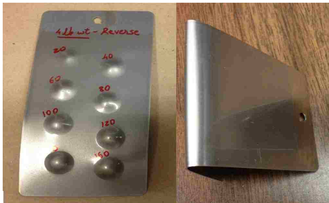
Figure 8. High impact resistance and flexibility of aziridine cured CUP clear coatings
