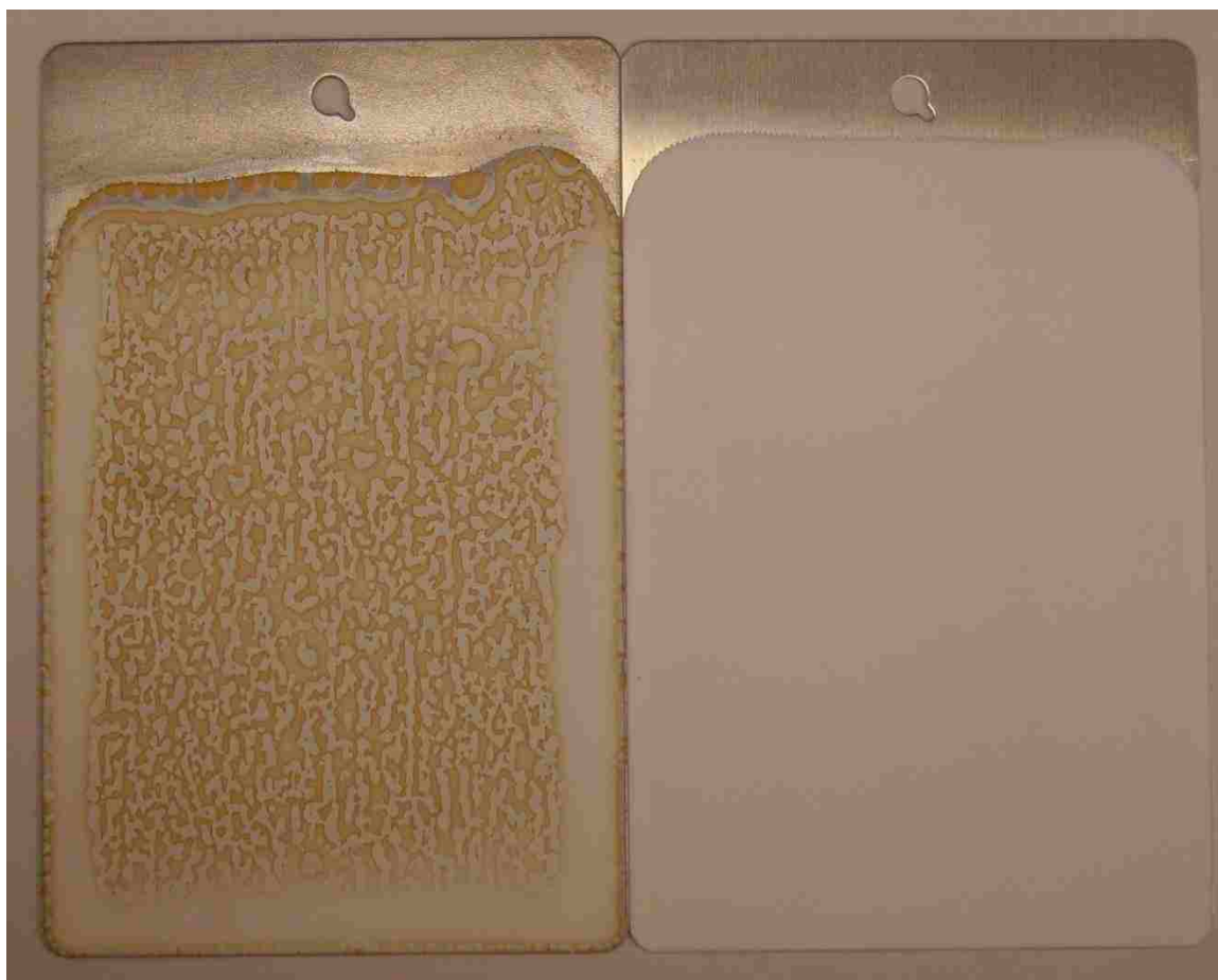
Figure 1. Flash rusting and staining patterns developed on paint films on steel panel without (left) and with (right) inhibitor H_2ADTZ
