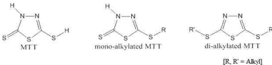
Figure 11. The results of X-ray crystallography, NMR spectroscopy and ab-initio electronic structure calculations indicate the preferred structures of MTT, mono-alkylated MTT and di-alkylated MTT.
