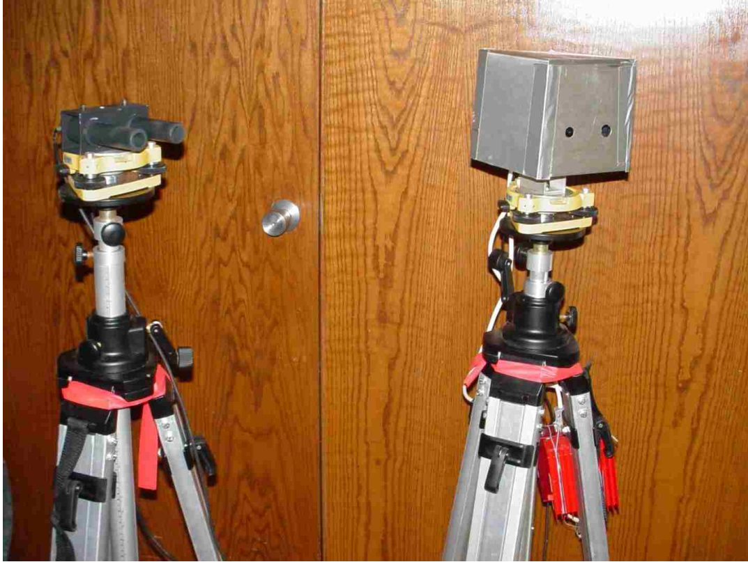
Figure 2.3 – Photograph of Laser Source and Detector Units Mounted on Field-Deployable Tripods
