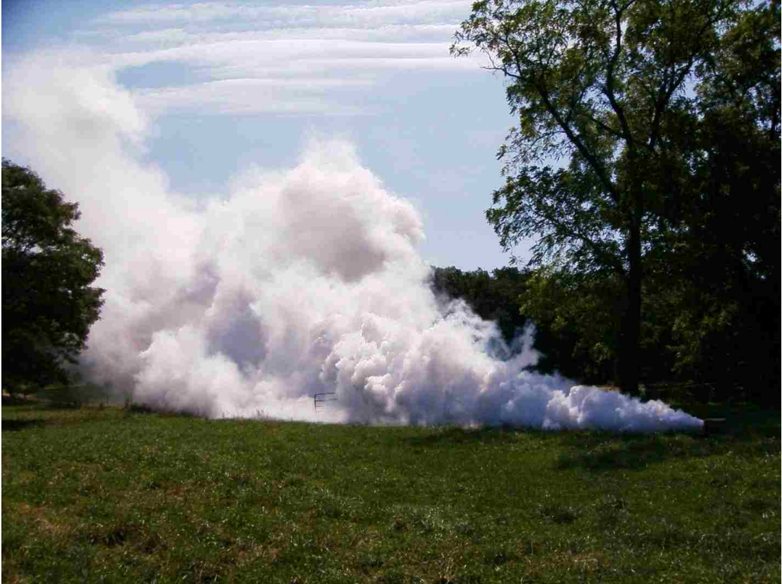
Figure 4.69 – Photograph of Demonstration of Methyl Soyate Plume from Prototype Modular Obscurant Aerosol Generator Remaining Dense and Near the Ground
