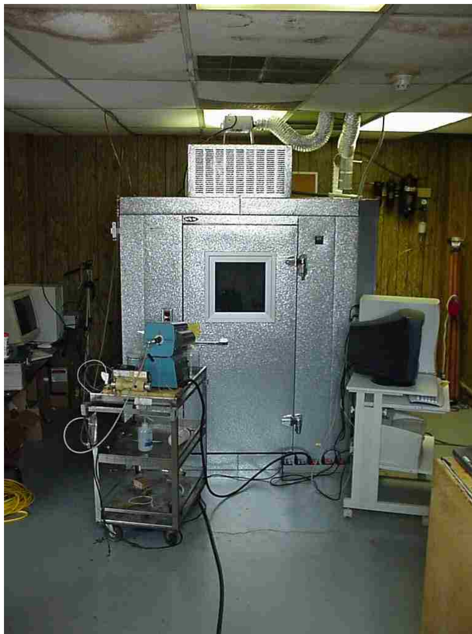
Figure 2.4 – Photograph of Laboratory Climate-Controlled Aerosol Testing Chamber with Tubular Furnace-Based Obscurant Aerosol Generator
