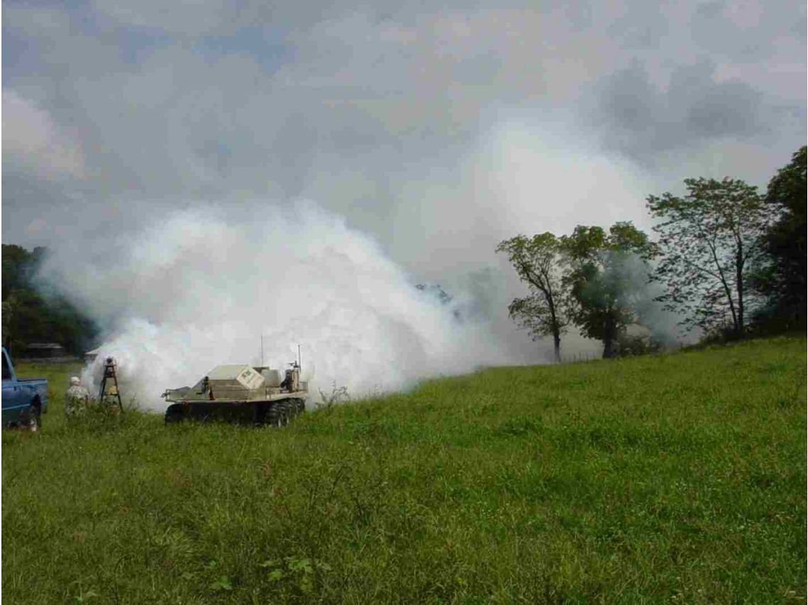
Figure 4.67 – Photograph of Simultaneous Obscuration by Prototype Modular Obscurant Aerosol Generator on Amphibious Vehicle and Exposed Obscurant Generator
