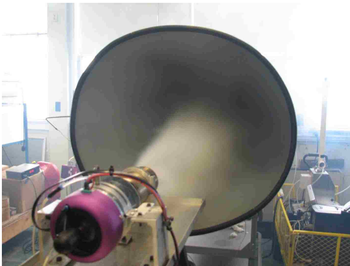
Figure 4.55 – Photograph of Obscurant Aerosol Passing Through the Laboratory High-Throughput Aerosol Characterization Facility
