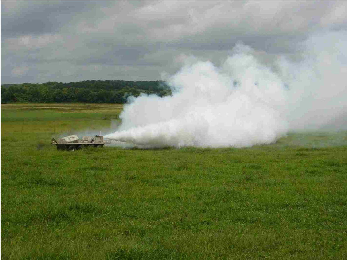
Figure 4.64 – Photograph of Radio Controlled Prototype Modular Obscurant Aerosol Generator Mounted to Radio Controlled Amphibious Vehicle
