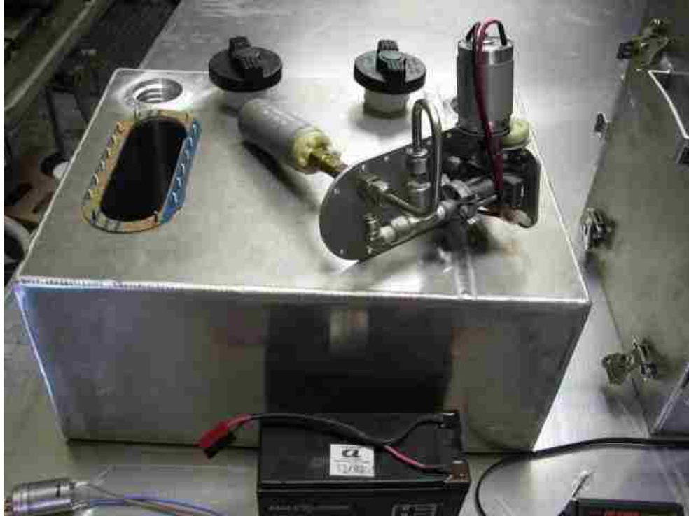
Figure 3.8 – Photograph of Early Design of Prototype Generator Fuel Tank with Single Nozzle Obscurant Sprayer Pump Assembly
