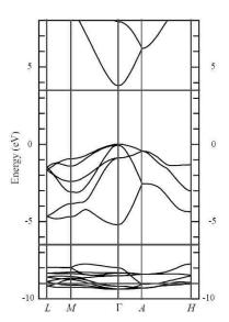
**Figure 1.2.** Local density approximation (LDA) band structure of bulk wurtzite ZnO in the hexagonal Brillouin zone calculated with dominant atomic self-interaction-corrected pseudopotentials (SIC-PP). <sup>31</sup>
