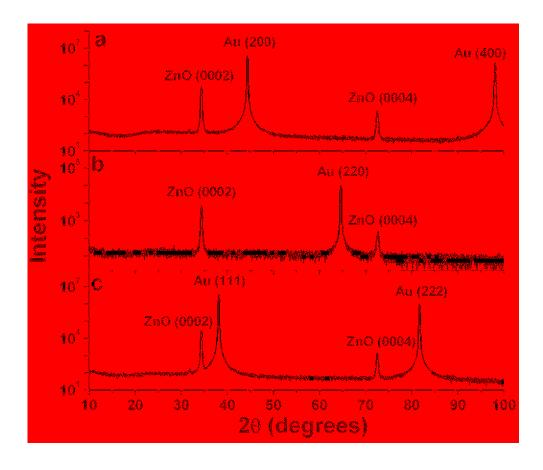
**Figure 11.** X-ray symmetric  $\theta$ -2 $\theta$  scans on the epitaxial ZnO deposited on the single crystal substrates of Au(100) (a), Au(110) (b) and Au(111) (c).
