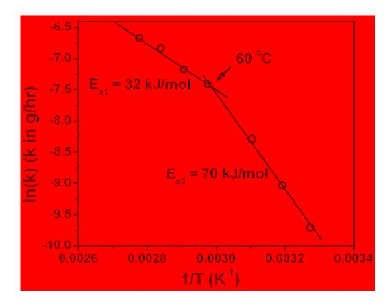
**Figure 5.** Arrhenius plot of the deposition process, ln(k) versus 1/T, where temperature (T) is in the unit of Kelvin and rate constant (k) is in the unit of  $\mu g/hr$ . The breakpoint is due to two different products (ZnO and  $\varepsilon$ -Zn(OH)<sub>2</sub>) that are deposited at the two side of this point.
