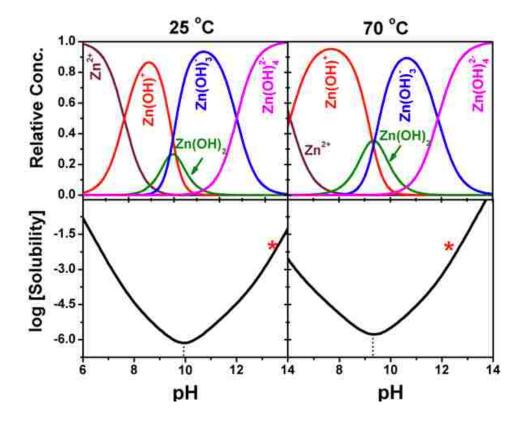
**Figure A.1.** Speciation distributions (upper) and solubility diagrams (lower) of Zn(II) versus pH in aqueous solution at 25  $^{\circ}$ C (left) and 70  $^{\circ}$ C (right). The asterisks represent the slightly oversaturated state of the deposition solution that contains 0.25 M NaOH and 8 mM Zn(NO<sub>3</sub>)<sub>2</sub>.
