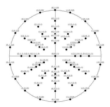
**Figure 1.10.** The (0001) stereographic projection of ZnO (hexagonal, a = 3.2498 Å, c = 5.2066 Å).
