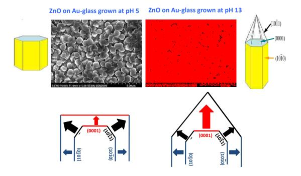
**Figure B.7.** SEM images of ZnO electrochemically deposited on Au coated microscope slides from acidic solution that contain  $0.1 \text{ M Zn}(NO_3)_2$  (top, left) and from alkaline solution that contain 0.25 M NaOH and  $8 \text{ mM Zn}(NO_3)_2$  (top, right), along with the illustrations showing the crystal growth habit.
