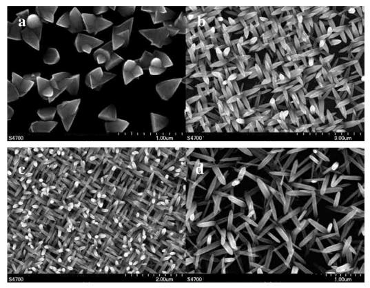
**Figure B.3.** ZnO chemically deposited on Si(001) substrates from solutions containing 0.25 M base and 8 mM Zn(NO<sub>3</sub>)<sub>2</sub> at 70 °C for 15 minute using different bases (a) LiOH, (b) NaOH, (c) KOH, and (d) CsOH.
