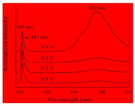
**Figure 4.** PL spectra of the films deposited on Au-glasses by applying deposition potentials of -0.1V, -0.2 V, -0.3 V, and -0.4 V versus Ag/AgCl. The intensity of each emission peak is normalized according to the maximum of the emission peak at 409 nm.
