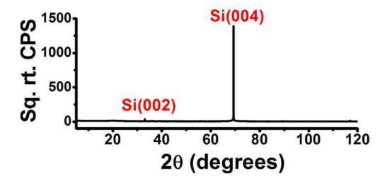
**Figure 3.** Symetric X-ray diffraction pattern on the as-deposited ZnO on the Si(001) substrate.
