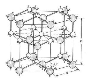
**Figure 1.1.** ZnO hexagonal wurtzite structure. The larger gray balls represent O atom, and the smaller white balls represent Zn atom.
