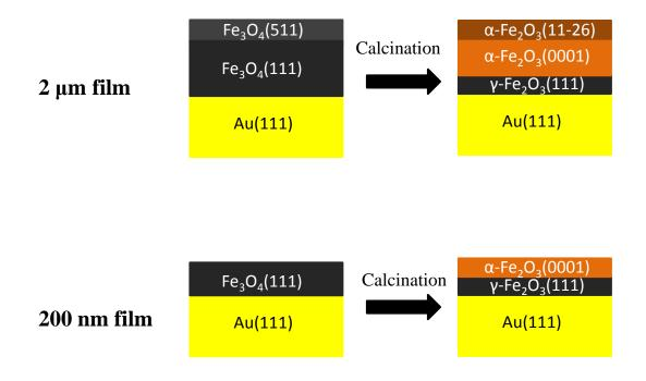
**Figure C.10.** Illustrations of the thermal transformation of the magnetite films (Fe<sub>3</sub>O<sub>4</sub>) as deposited on single crystalline Au(111) substrate at -1.065 V versus Ag/AgCl until 0.1 C/cm<sup>2</sup> (200 nm) and 0.1 C/cm<sup>2</sup> (2  $\mu$ m). The film is annealed in O<sub>2</sub> atmosphere at 400 °C for 4 hours.
