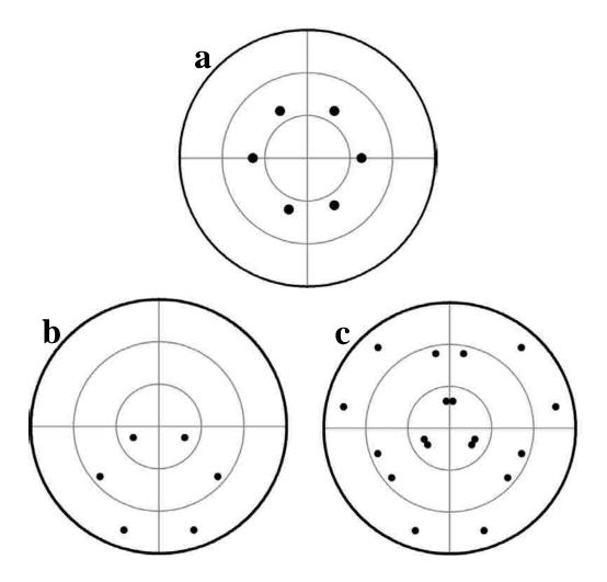
**Figure C.4.** Stereographic projection with hematite (1014) type reflection. (a) with (0001) out-of-plane orientation, 6 spots are found at  $38.24^{\circ}$ . (b) with (1126) out-of-plane orientation, 2 spots are found at  $19.66^{\circ}$ , 2 are at  $54.48^{\circ}$ , another 2 are at  $77.28^{\circ}$ . (c) the resulting stereographic projection after rotating the stereographic projection in (b) by  $120^{\circ}$  and  $240^{\circ}$ , then overlaying each other.
