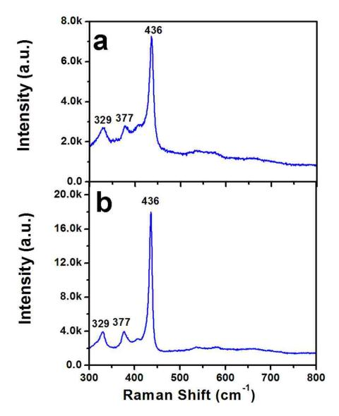
**Figure 8.** Raman spectra on the ZnO as deposited on polycrystalline Pt (a) and after calcination at °C for 1 hour (b).
