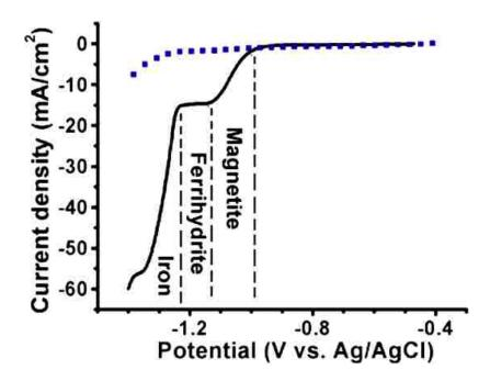
**Figure C.1.** Linear sweep voltammograms of an alkaline TEA solution (blue squares) and Fe(III)-TEA solution (black solid line) at 80 °C scanned at 50 mV/s at a rotation of 100 rpm on a gold rotating disk electrode. The alkaline TEA solution consisted of 0.1 M TEA in 2 M NaOH. The alkaline Fe(III)-TEA solution consisted of 43 mM Fe<sub>2</sub>SO<sub>4</sub>, 0.1M TEA, and 2M NaOH.
