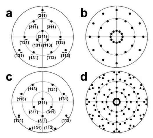
**Figure 7.** The (111) (a) and (511) (c) stereographic projections of CuI probing (311)-type reflections. Rotating (a) and (c) by  $0^{\circ}$ ,  $90^{\circ}$ ,  $180^{\circ}$ , and  $270^{\circ}$  and then overlaying the four rotating images results the stereographic projections in (b) and (d) respectively, which are consistent with the pole figures in Figure 6 (a) and (b).
