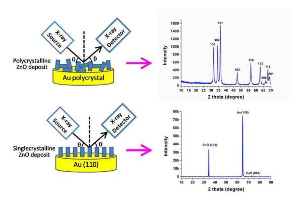
**Figure 1.7.** Setup (left) used to acquire X-ray diffraction patterns, and the resulting XRD patterns of a polycrystalline zinc oxide film (right, upper) deposited on an Au-sputtered microslide substrate and a epitaxial zinc oxide film (right, lower) deposited on an Au(110) single crystalline substrate. Both films were deposited by chemical bath deposition method from a solution containing 0.25 M of NaOH and 10 mM of Zn(NO<sub>3</sub>)<sub>2</sub> at 70 °C for 30 minutes.
