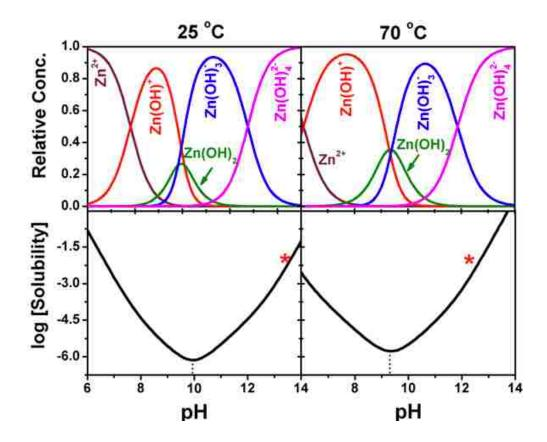
**Figure 1.** Speciation distributions (upper) and solubility diagrams (lower) of Zn(II) versus pH in aqueous solution at 25  $^{\circ}$ C (left) and 70  $^{\circ}$ C (right), asterisks representing the slightly oversaturated state of the deposition solution that contains 0.25 M NaOH and 8 mM Zn(NO<sub>3</sub>)<sub>2</sub>.
