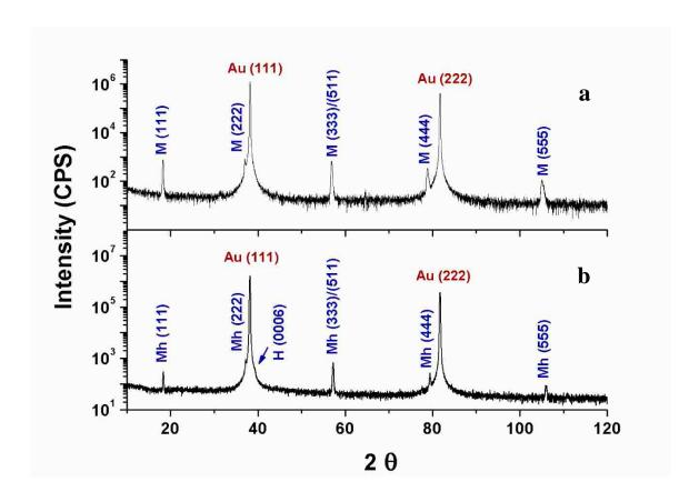
**Figure C.5.** Symmetric X-ray diffraction patterns of the magnetite film (Fe<sub>3</sub>O<sub>4</sub>) as deposited (a) and after calcination (b) in an O<sub>2</sub> atmosphere at 400  $^{\circ}$ C for 4 hours. The magnetite is deposited on single crystalline Au(111) substrate at -1.065 V versus Ag/AgCl until 0.1 C/cm<sup>2</sup> was passed. The film is estimated to be 200 nm thick.
