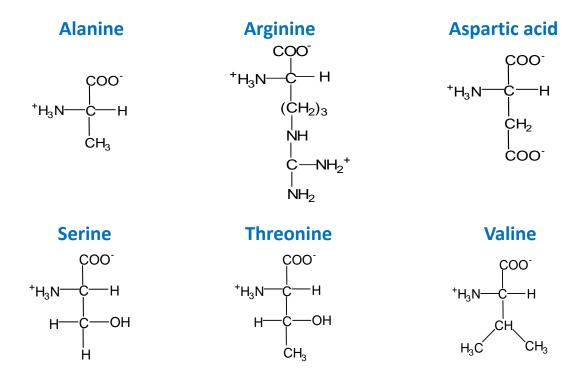
**Figure B.4.** Six different amino acids that can be used to be electroxidized to generate proton in the alkaline solutions for ZnO deposition: alanine, arginine, aspartic acid, serine, threonine, and valine.
