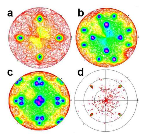
**Figure 4.** (a) (0001), (b)(10 $\overline{1}0$ ), and (c) (10 $\overline{1}1$ ) pole figures for ZnO and (d) (111) pole figure for the Si(001) substrate. The radial grid lines on each pole figure correspond to 300 increments in  $\chi$ .
