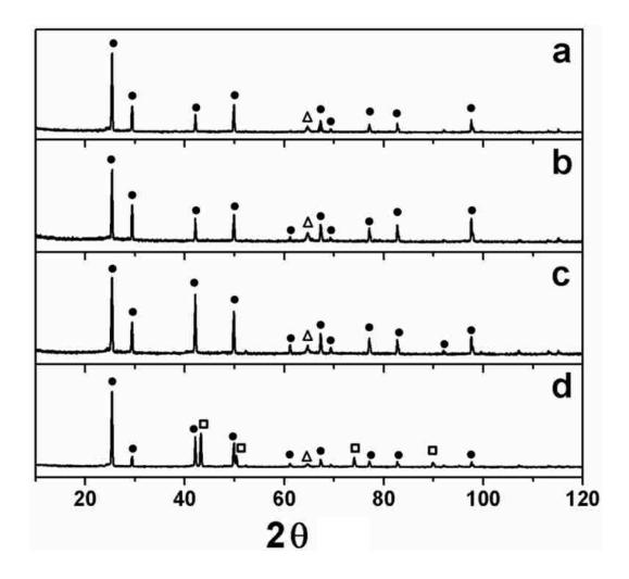
**Figure 2.** X-ray diffraction symmetric scans of the films deposited on Au coated microscope slides at -0.1V (a), -0.2 V (b), -0.3 V (c), and -0.4 V (d) versus Ag/AgCl. The solid circles represent the X-ray diffraction peaks for CuI, the hollow triangles represent the peaks for Au, and the hollow squares represent the peaks for Cu.
