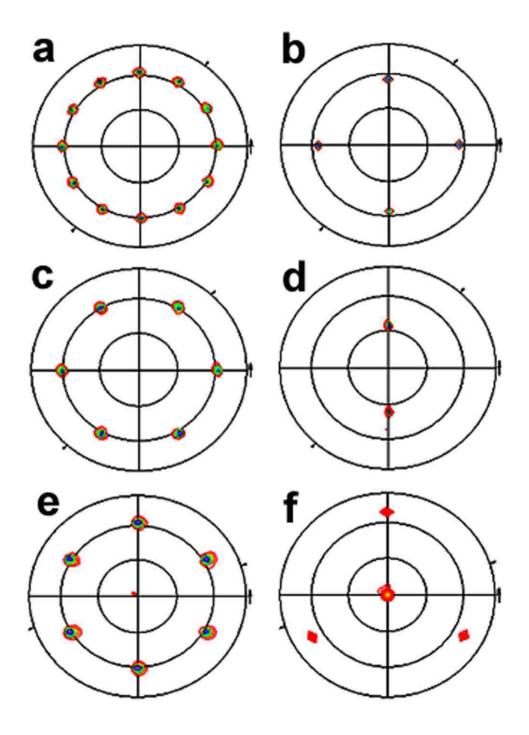
**Figure 12.** ZnO ( $[0\overline{1}]$ ) pole figures on the ZnO deposited on the single crystal substrates of Au(100) (a), Au(110) (c) and Au(111) (e), as well as the corresponding Au(111) substrate pole figures for Au (100) (b), Au(110) (d) and Au(111) (f) substrates. The radial grid lines on each pole figure correspond to 30° increments in  $\chi$ .
