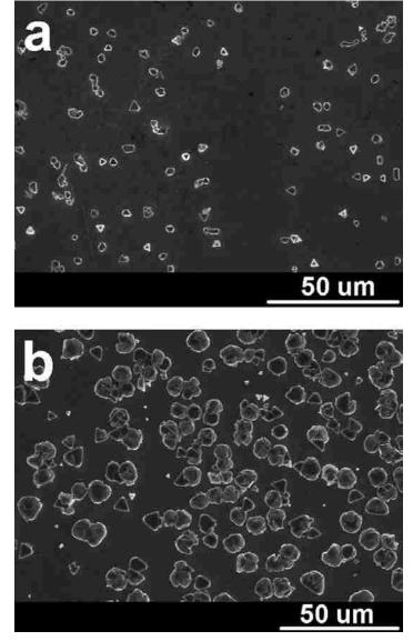
**Figure 8.** SEM images of the CuI films on Au(100) substrate to charge density  $0.1 \text{ C/cm}^2$  (a) and  $0.5 \text{ C/cm}^2$  (b).
