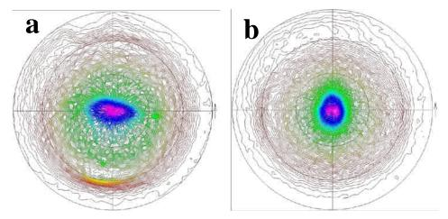
**Figure C.16.** X-ray pole figures of the ferrihydrite films on Au(110) substrate before (a) and after (b) annealing in  $O_2$  at 400 °C for 4 hours. (a) is a ferrihydirte (110) pole figure. (b) is a hematite (1120) pole figure.
