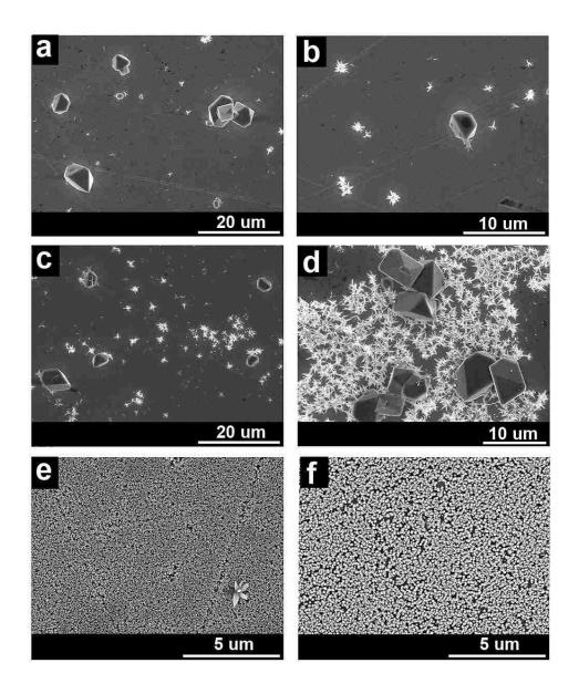
**Figure 3.** SEM micrographs of the deposits on Au-glass substrates grown at 30  $^{\circ}$ C (a), 40  $^{\circ}$ C (b), 50  $^{\circ}$ C (c), 55  $^{\circ}$ C (d), 60  $^{\circ}$ C (e), and 70  $^{\circ}$ C (f). The large orthorhombic crystals are  $\varepsilon$ -Zn(OH)<sub>2</sub> crystals, and the smaller hexagonal nanocolumns are ZnO.
