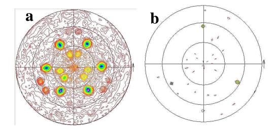
**Figure C.3.** The  $(10\overline{1}4)$  pole figure of hematite (a) on the magnetite film after calcination in an  $O_2$  atmosphere at 400 °C for 4 hours, and the Au(100) substrate pole figure (b) on Au(111) single crystalline substrate. The magnetite was electrodeposited on single crystalline Au(111) substrate at -1.065 V versus Ag/AgCl until 1 C/cm<sup>2</sup> was passed. The film is estimated to be 2  $\mu$ m thick.
