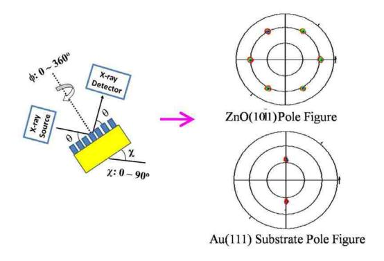
**Figure 1.8.** Setup used to acquire X-ray pole figure (left) and the resulting pole figures for a (0001) oriented zinc oxide film (right, upper) deposited on Au(110) single crystalline substrate and its correspondent substrate pole figure (right, lower). The ZnO was deposited by chemical bath deposition method from a solution containing 0.25 M of NaOH and 10 mM of Zn(NO<sub>3</sub>)<sub>2</sub> at 70 °C for 30 minutes.
