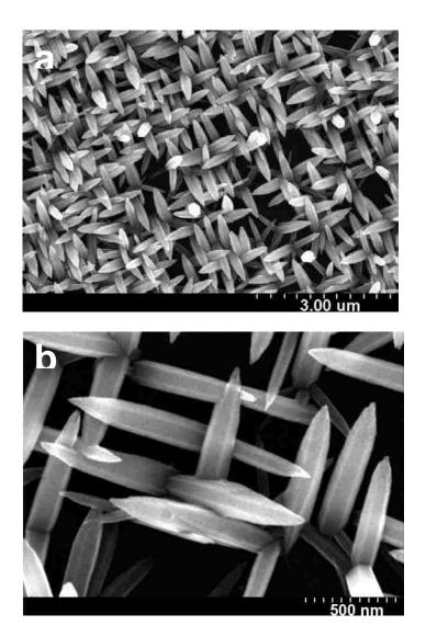
**Figure 2.** SEM images of as-deposited ZnO on the Si(001) substrate. (a) low- (bar marker = 3 um), and (b) high-magnification (bar marker = 500 nm) images.
