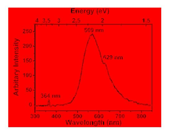
**Figure 8.** Room temperature PL spectrum of as-deposited ZnO, using an  $Ar^+$  ion laser ( $\lambda = 355$  nm) as the excitation source.
