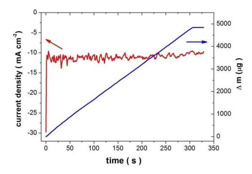
**Figure C.11.** EQCM study on the electrodeposition of ferrihydrite. Red line is the recoding current, blue line the mass increase on the EQCM electrode. The ferrihydrite is deposited on the Au coated side of the electrodeposited at -1.200 V versus Ag/AgCl from Fe(III)-TEA solution.
