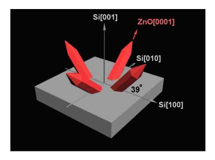
**Figure 6.** Schematic of the epitaxial  $ZnO(20\overline{23})$  nanospears on Si(001) substrate. The red spears on the top represent ZnO, whereas the grey base represents Si.
