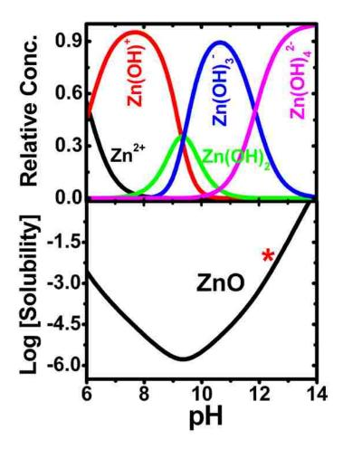
**Figure 1.** Speciation distribution (upper) and solubility (lower) of Zn(II) versus pH in aqueous solution at 70 °C. The asterisk represents the slightly supersaturated state of the deposition solution containing 6.0 mM of  $Zn(NO_3)_2$  and 0.25 M NaOH.
