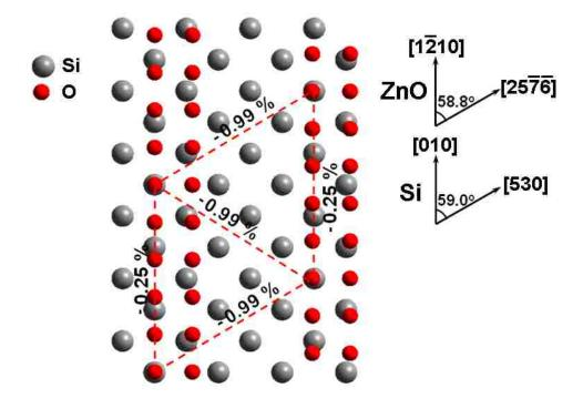
**Figure 7.** Interface model for the  $ZnO(20\overline{2}3)$  on Si(001) planes. The Si atoms are gray, and the O atoms are red. Based on this model, the lattice mismatch is reduced from - 40.16% to -0.25% in the  $ZnO\left[1\overline{2}10\right]$  in-plane direction and -0.99% in  $ZnO\left[25\overline{7}6\right]$  in-plane direction by tilting the nanospears  $51^\circ$  relative to the surface normal.
