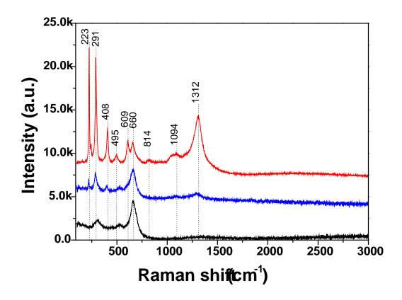
**Figure C.9.** Raman spectra of the magnetite films (Fe<sub>3</sub>O<sub>4</sub>) as-deposited on single crystalline Au(111) substrate at -1.065 V versus Ag/AgCl until 0.1 C/cm<sup>2</sup> (black line, bottom) and the same film after calcination in O<sub>2</sub> atmosphere at 400  $^{\circ}$ C for 4 hours (blue line, middle), and the 1 C/cm<sup>2</sup> film after calcination (red line, top).
