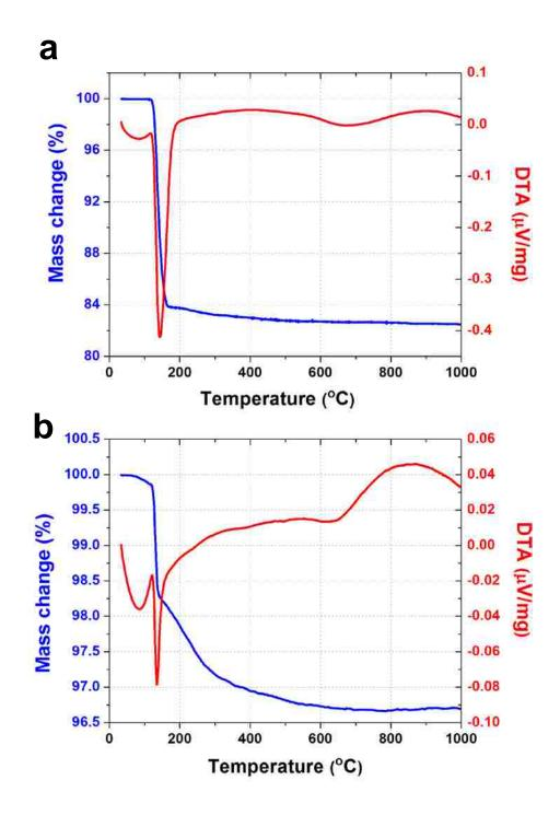
**Figure 7.** Thermogravimetry (TG) and differential thermal analysis (DTA) on the powders collected at  $40\,^{\circ}\text{C}$  (a) and  $70\,^{\circ}\text{C}$  (b), which were carried out in air environment, temperature increasing from 25 to 1,000  $^{\circ}\text{C}$  at a rate of  $10\,^{\circ}\text{C/min}$ .
