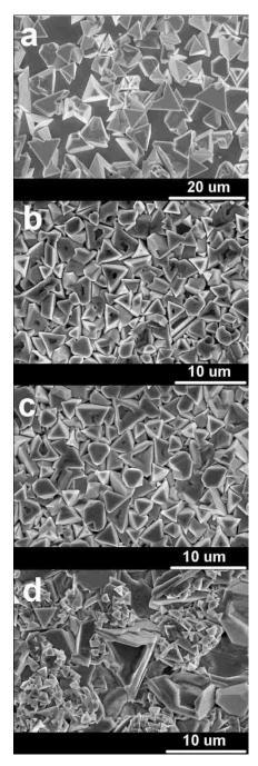
Figure 3. SEM images of the films deposited on Au-glasses at -0.1V (a), -0.2 V (b), -0.3 V (c), and -0.4 V (d) versus Ag/AgCl.
