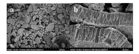
**Figure C.13.** SEM images of multiple electrodeposited ferrihydrite films (a) that were peeled offfrom the Au-glass substrate, and (b) annealed in  $O_2$  at 400  $^{\circ}$ C for 4 hours.
