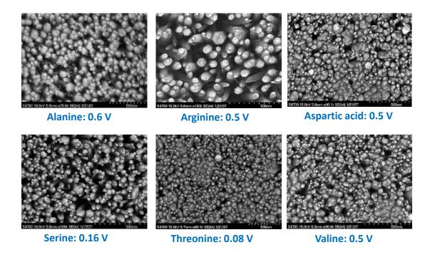
Fighthe Been siting potentials from referred to the Ass/Ass/Classical and Asserted Areference electroscope slides from solutions containing 0.25 M base, 5 mM Zn(NO<sub>3</sub>)<sub>2</sub> and 10 mM amino acids (alanine, arginine, aspartic acid, serine, threonine, and valine) at 70 °C for 15 minute. The constant potential versus Ag/AgCl applied for deposition is as shown under each image.
