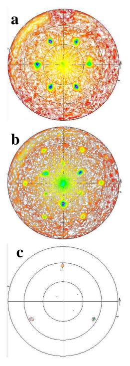
**Figure C.7.** The  $(10\overline{1}4)$  pole figure of hematite (a) and the (311) pole figure of maghemite on the magnetite film after calcination in  $O_2$  atmosphere at 400 °C for 4 hours, and the Au(100) substrate pole figure (b) on Au(111) single crystalline substrate. The magnetite is electrodeposited on single crystalline Au(111) substrate at -1.065 V versus Ag/AgCl until 0.1 C/cm<sup>2</sup> was passed. The film is estimated to be 200 nm thick.
