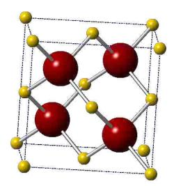
**Figure 1.4.** A unit cell of the zinc blende  $\gamma$ -CuI crystal structure. The larger red balls represent I atoms, and the smaller yellow balls represent Cu atoms.
