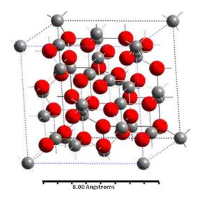
**Figure 1.6.** A unit cell of magnetite (Fe<sub>3</sub>O<sub>4</sub>) with an inverse spinel structure, space group  $Fd\overline{3}m$ .
