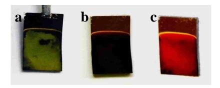
**Figure C.12.** Photo images of the three samples deposited on Au coated microscope slides. (a) is the film immediately taken out from the deposition solution. (b) is the (a) film exposed to air for 5 minutes, (c) is the same film after being air dried for 2 hours.
