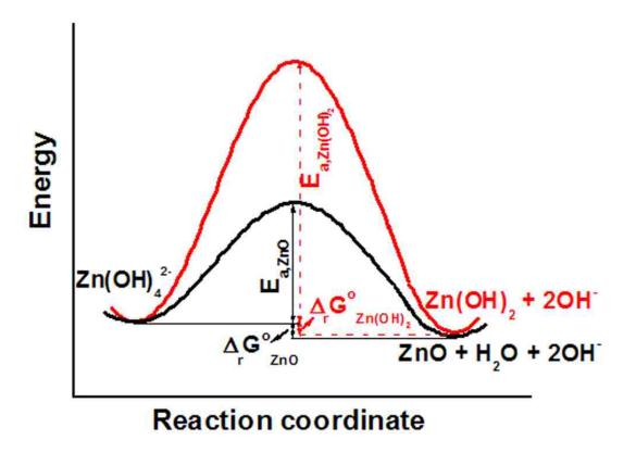
Figure 6. Overall reaction coordinates of the chemical bath deposition processes considering both ZnO and  $\epsilon$ -Zn(OH)<sub>2</sub> as products.
