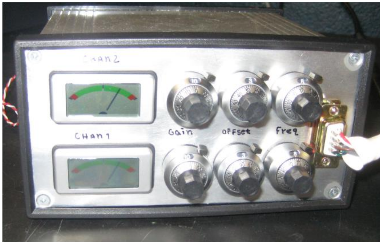
Figure 6.4 Conductivity System Set-up. Monitors changes in the solution's conductivity across the detection area between the electrodes. The system supplies an AC current of \pm 5 \mu\text{A} at \sim 40 \text{ kHz} to avoid charge build up at the electrode surfaces due to C_d . This system is capable of monitoring events at the first dimension (CHAN 1) and second dimension (CHAN 2).
