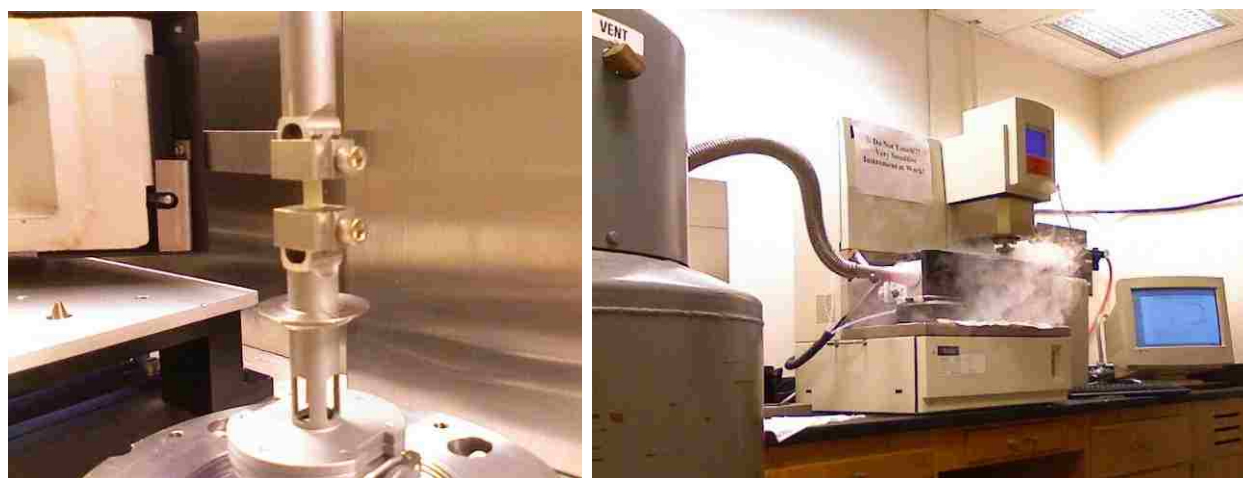
Figure 4.2: ARES instrument (right), equipped with a torsional tool (left), a heating oven and a liquid nitrogen controller, performing DMA measurements on nanocomposite thin films at negative temperatures.
