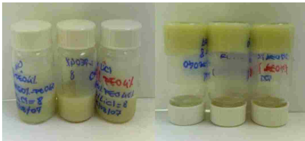
Figure 3.2: A picture showing the 3 vials containing the CNA6%-PEO4% dispersions before (left) and after (right) inversion. As observed on the right, at rest all gels are self supporting (no flow even after 24 hours)
