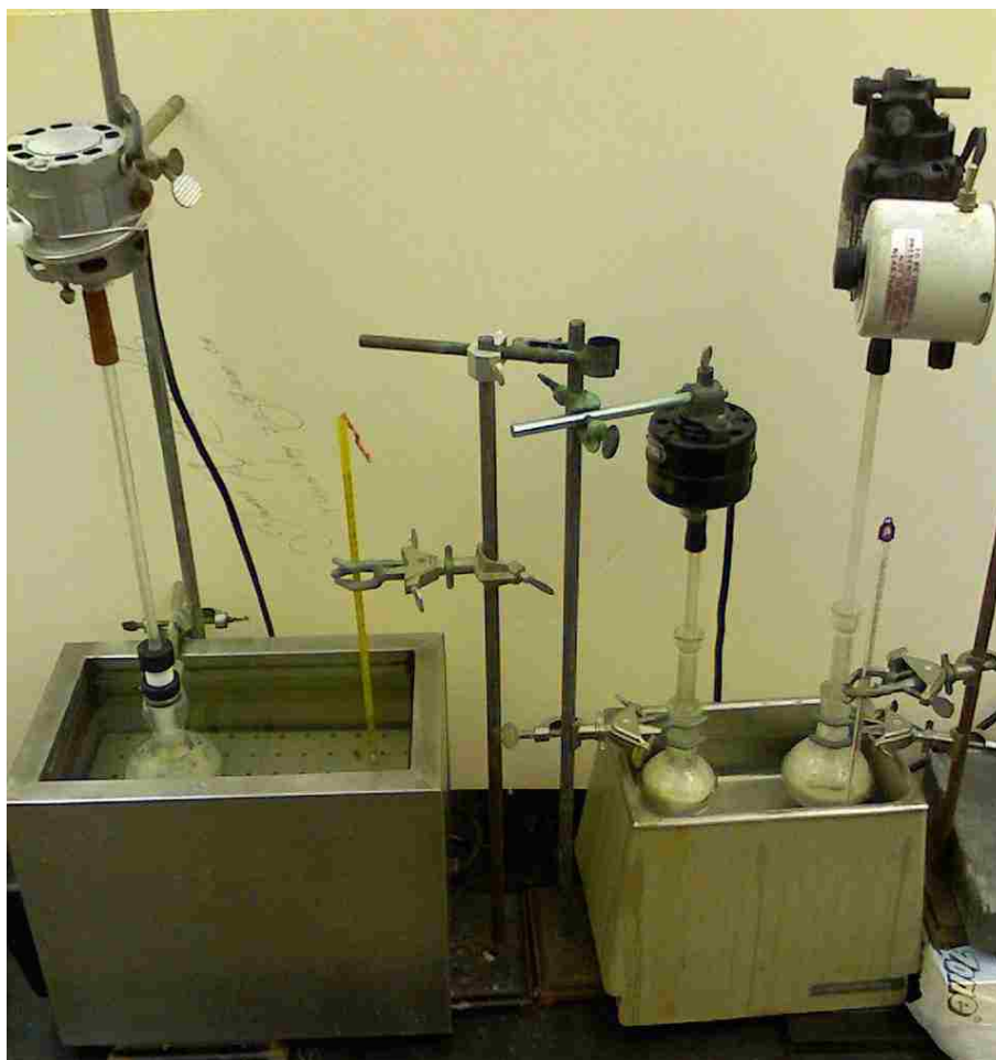
Figure 3.1: The setup used for the preparation of CNA6%-PEO4% dispersions. The three round bottom flasks are immersed in two water baths, of which temperature is recorded using mercury thermometers. On top of each flask there is an overhead mixer.
