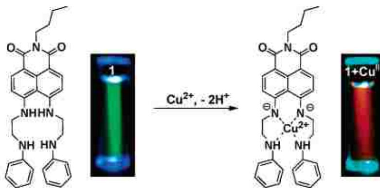
Figure 1.11. Binding of \text{Cu}^{2+} and deprotonation of the two aromatic amines. From Xu et al. (2005). 130
