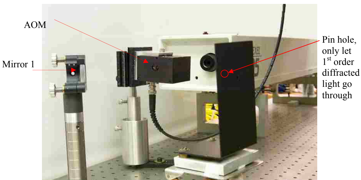
Figure 4.13 Close view of AOM, pinhole and mirror.
