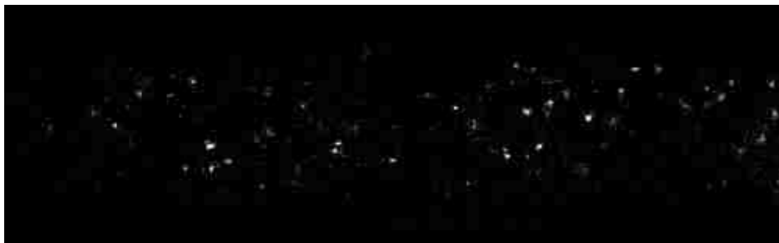
Figure 6. Yoyo-I labeled lambda-DNA molecules imaged one by one by fluorescence microscopy using a square capillary.
