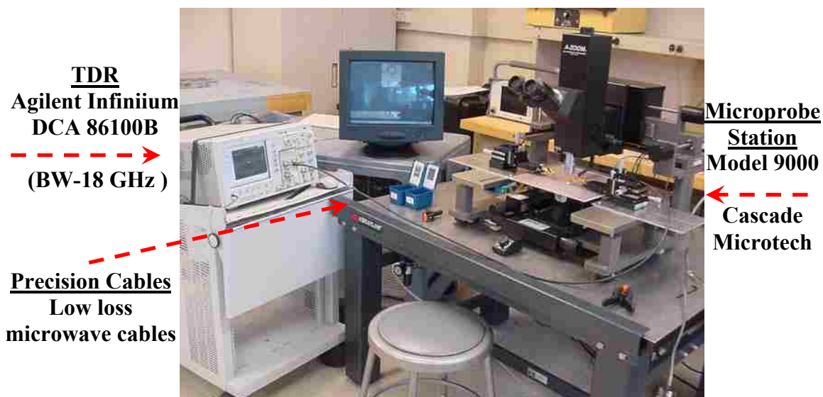
Figure 2.32. Test setup used for TDR measurements on microstrip test boards.
