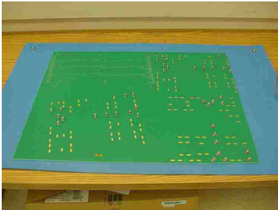
Figure 2.4. Perspective view of the stripline test board.
