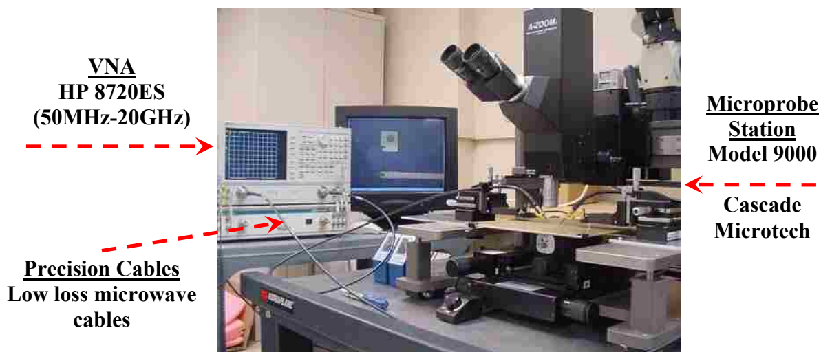
Figure 2.25. Test setup for microstrip test board measurement.
