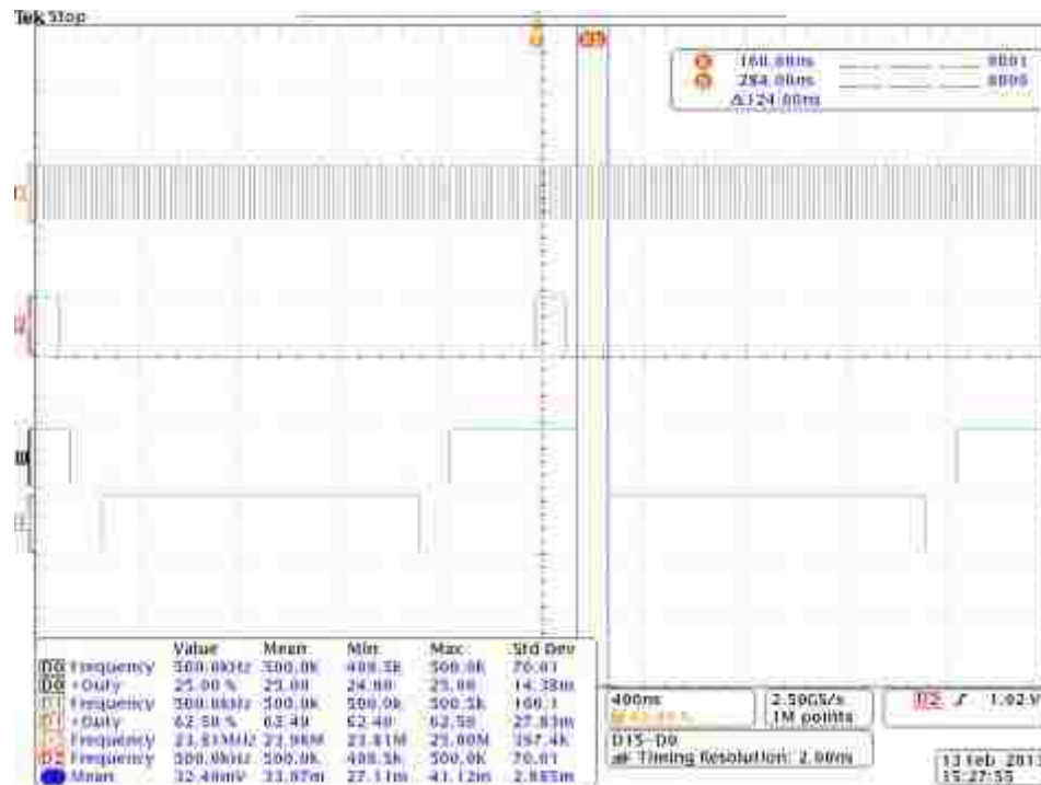
Figure 5.7 Dead Time of 124ns between the Two Gate Signals
