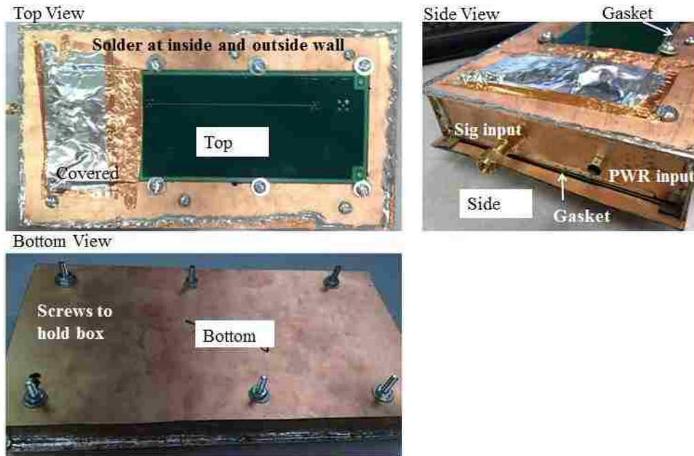
Figure 5.4. Different views of the shield box
