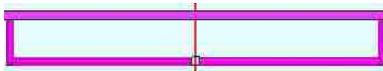
Fig. 3.12 Magnetic dipole approximated with a small loop antenna.
