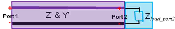
Fig. 2.11. A simplified model using an equivalent transmission line with terminations for both single-ended and differential cases. For differential cases, the reference plane is omitted
