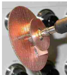
Figure 5.11. The perforated disk resonator stub used in measurements. (a) Side view of the perforated disk resonator stub. (b) Actual measurement setup of the perforated disk resonator stub (c) Coax launch model for the perforated disk resonator stub in HFSS.
