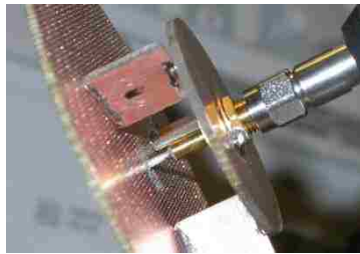
Figure 5.2. The solid disk resonator stub used in measurements. (a) Side view of the solid disk resonator stub used in the measurements. (b) Actual measurement setup of the solid disk resonator stub. (c) Coax launch model for the solid disk resonator stub in HFSS.
