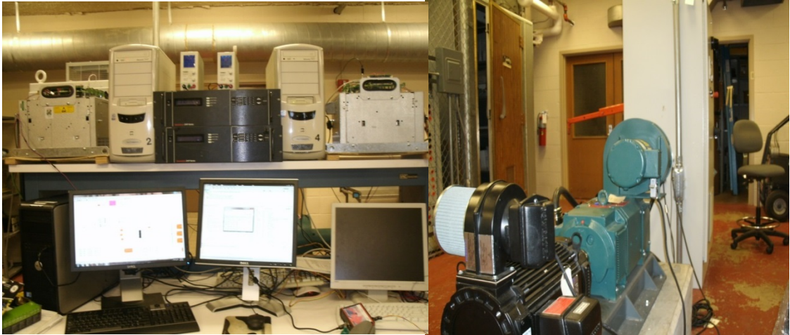
Figure 4.10. Lab set up for efficient and stabilized V/f for PMSM machine
