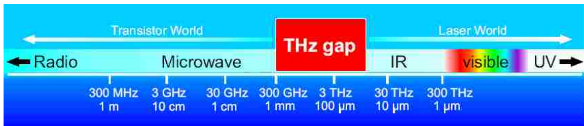
Figure 2.1 The THz gap in the electromagnetic spectrum [15]
